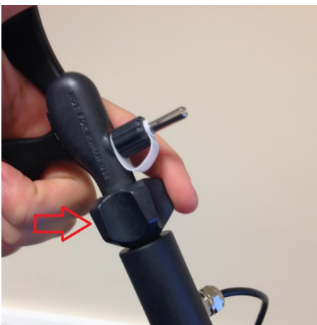
Figure 30: Cogwheel for rotation of instrument tips
