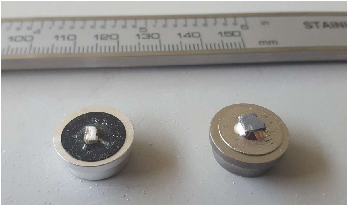
Figure 3-32 – SEM Kaolin sample mounted on holder using epoxy (L) and after sputter coating (R)
