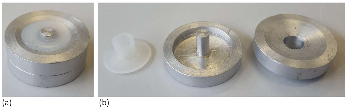
Figure 3-15 – (a) Thermoplastic EVA grommet for mid-height PPT and (b) two-part aluminium mould
