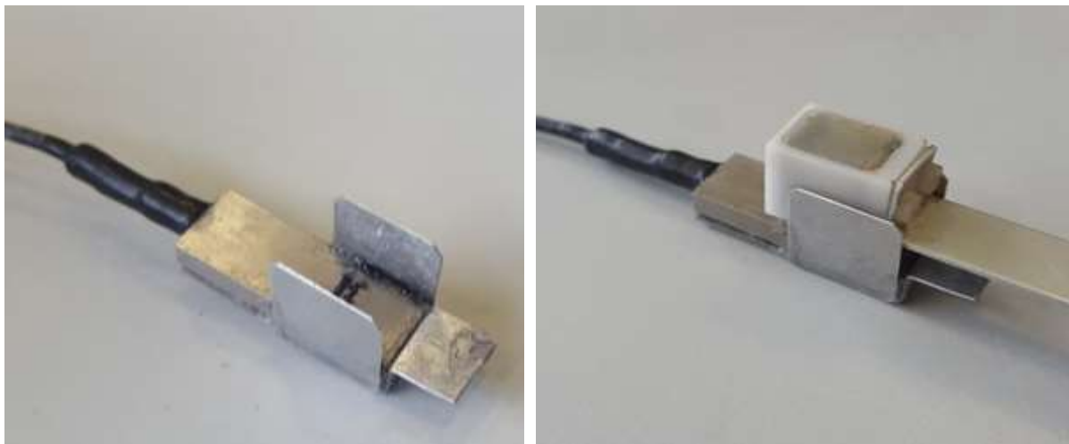
Figure 3-13 – Axial Hall effect transducer with the modified aluminium extension fins (with and without magnet)
