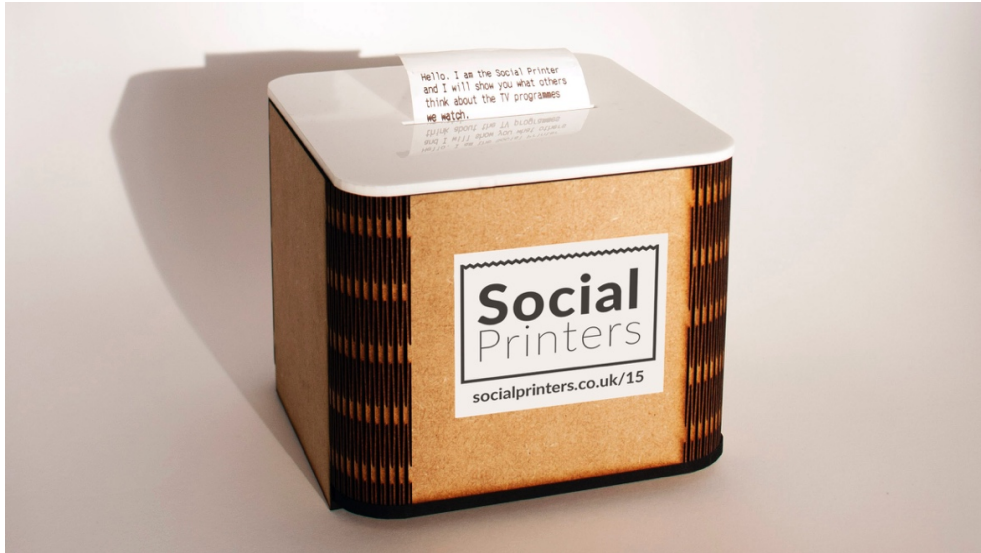
Figure 15 The Social Printer was essentially a small laser-cut box containing an Electric Imp and a thermal printer.
