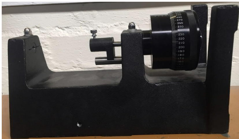
Figure A.1. Extensometer calibrator used for calibration of the LVDT
