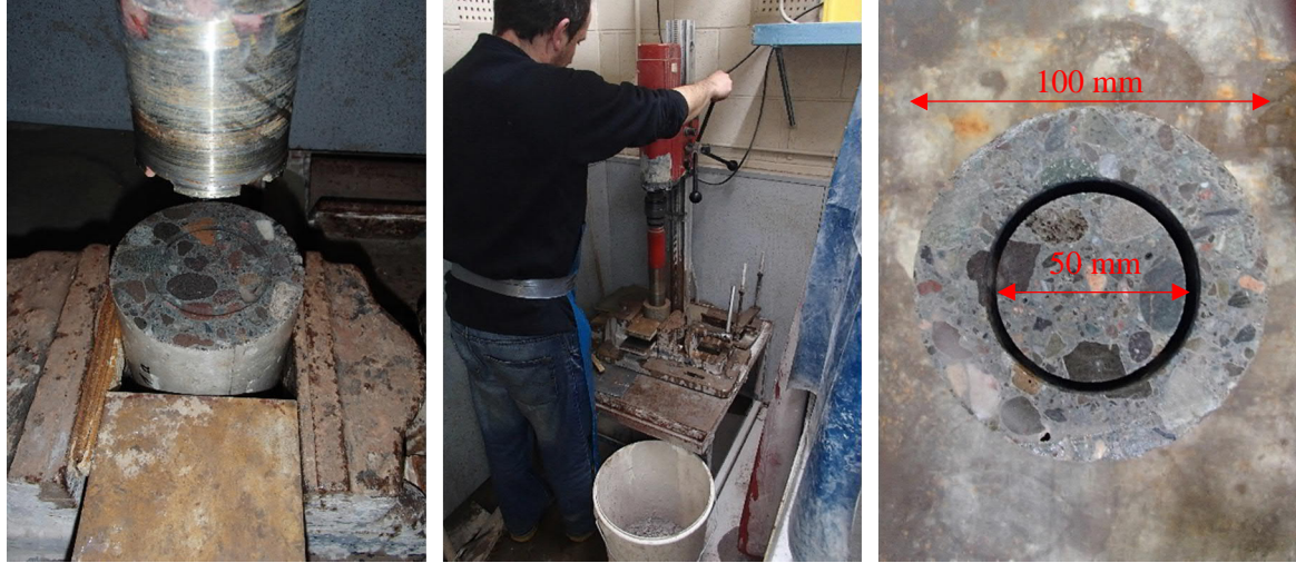
Figure 3.18. Torsion test: preparation of circular sections
