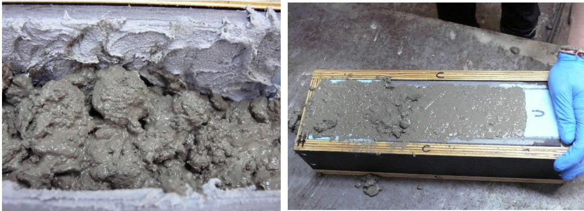
Figure 3.23. Fresh concrete casting with epoxy for double lap shear test
