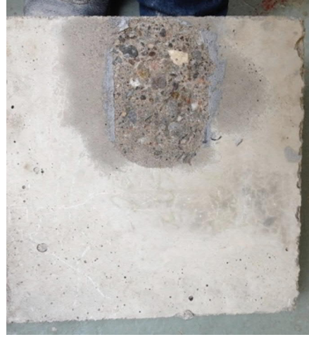
Figure 4.16. Failure mode in push out test without any paint on the steel
