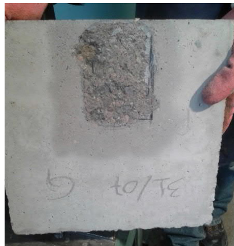
Figure 4.18. Failure mode in push out test with the epoxy anti-corrosion paint on steel
