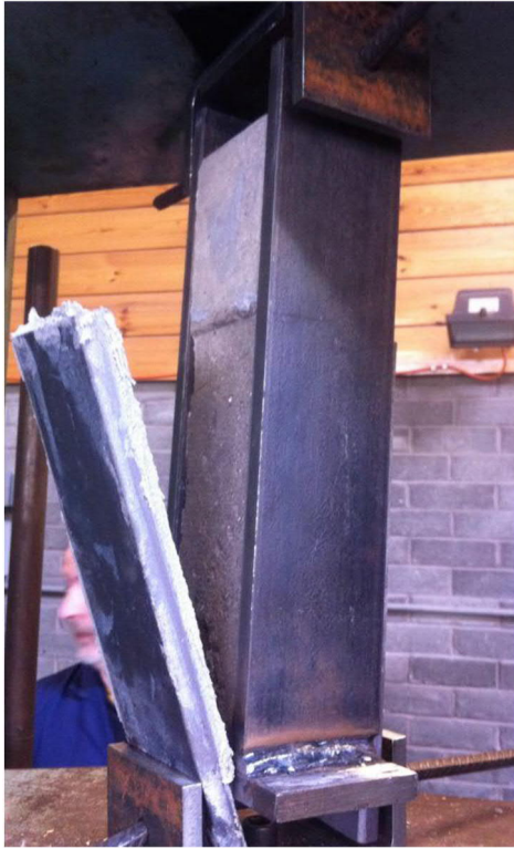
Figure 4.20. Failure mode of bonded hard concrete to steel
