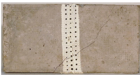
(a) Cohesive failure in specimen T2
