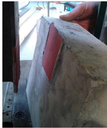
Figure 4.17. Failure mode in push out test with the normal anti-corrosion paint on the steel
