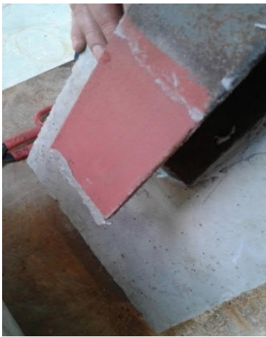
Figure 4.17. Failure mode in push out test with the normal anti-corrosion paint on the steel
