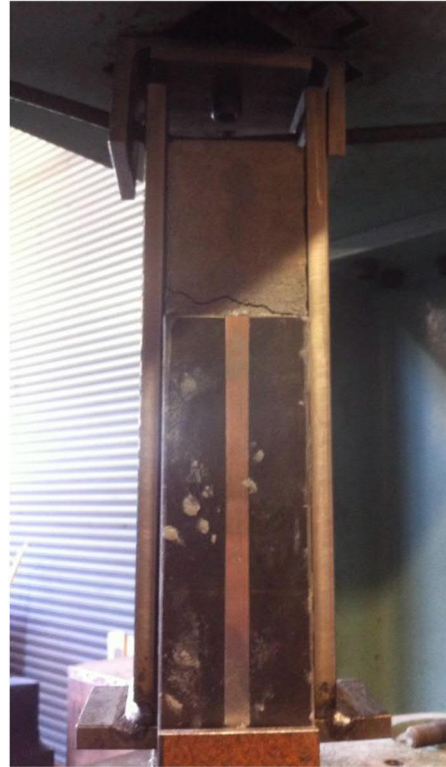
Figure 4.20. Failure mode of bonded hard concrete to steel
