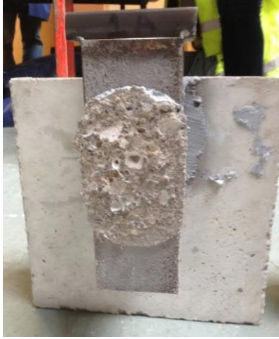
Figure 4.16. Failure mode in push out test without any paint on the steel
