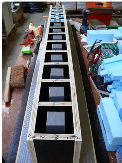
(a) Wooden mould with the spacers
