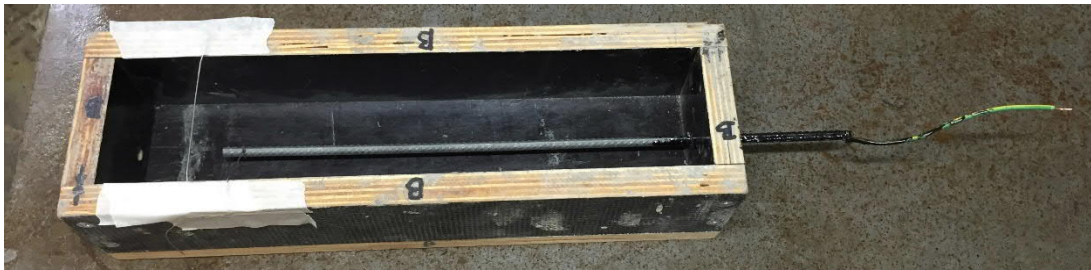
Figure 3.36. Mould, 6 mm rebar, and connection wire
