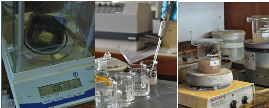
Figure B.1. Acid soluble process using 5 M HNO 3
