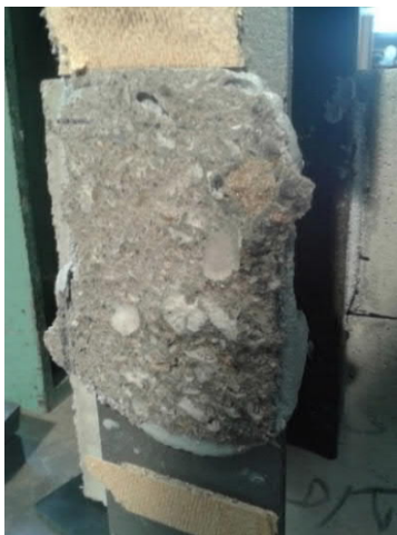
Figure 4.18. Failure mode in push out test with the epoxy anti-corrosion paint on steel
