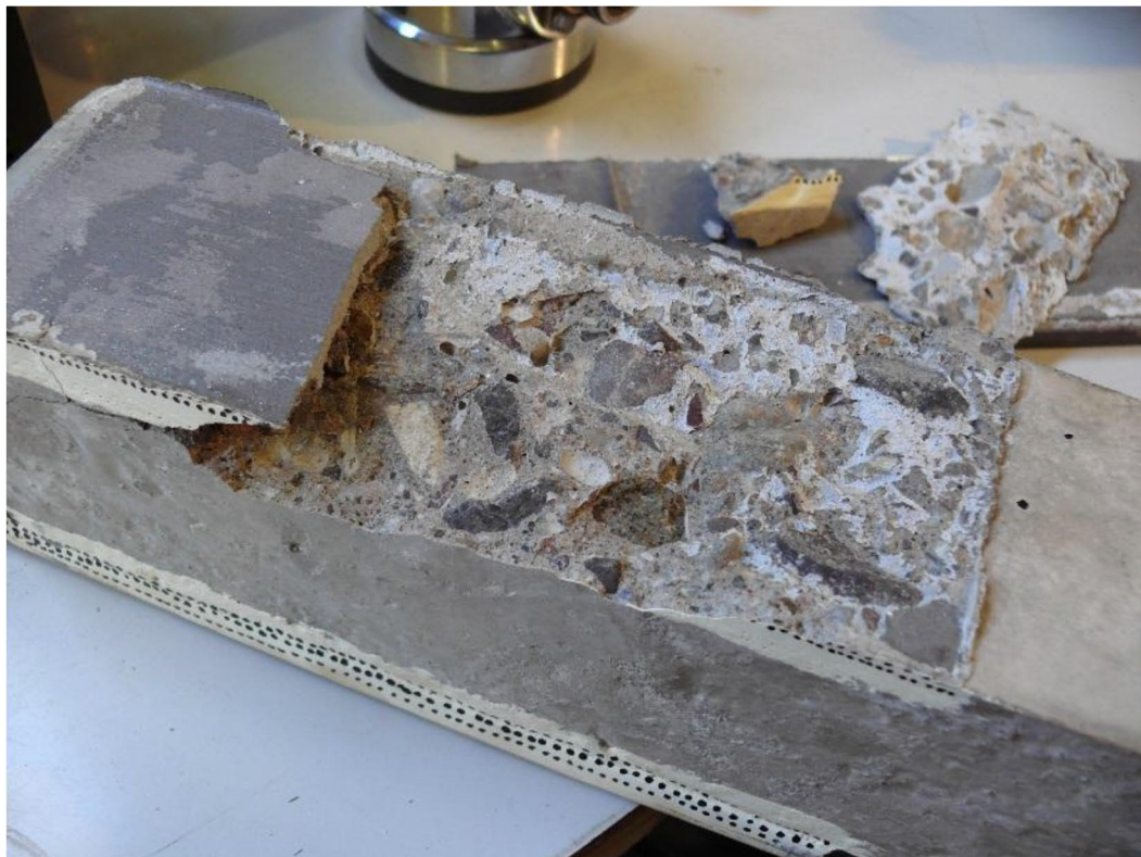
Figure 4.20. Failure mode of bonded hard concrete to steel
