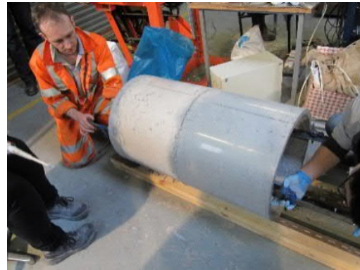
d) Applying temporary post-tensioning
