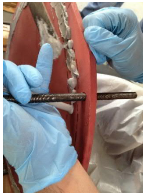
f) Applying epoxy
