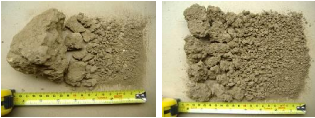
Fig 4.24. Examples of the results of subjecting aggregates to the soil structure and consistency drop test that forms part of the VSA. Left: field soil, right: pot soil.
