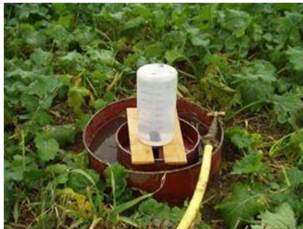
Fig. 4.2. Double ring infiltrometer used in December 2005 at Colworth on each of the fields shown in Fig. 4.1.
