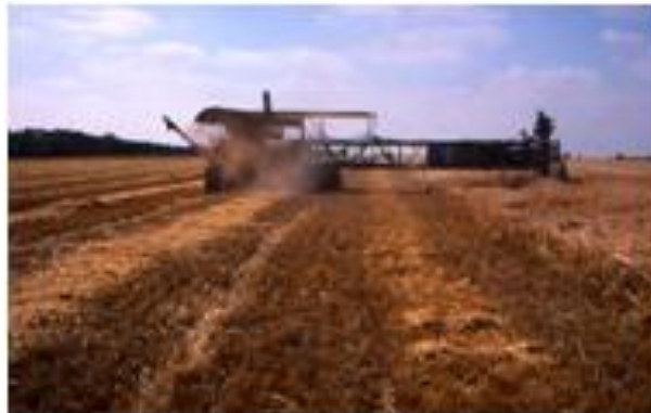
Fig. 2.9. A three drum and concave threshing and initial separation unit (Metianu, et al., 1990) were the basis of grain harvesting with this 12 m experimental gantry at Silsoe in the early 1990s.
