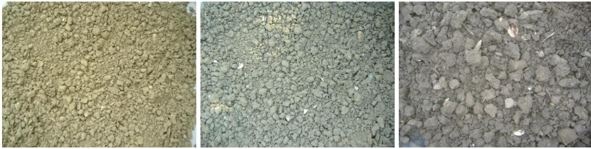
Fig. 4.22. Series of photos (left to right) taken on 29 th June, 2 nd July and 9 th July 2006 during which there were four wetting and drying cycles of the soil from Normanton Lodge.
