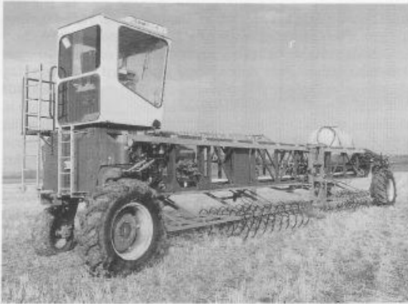
Fig. 1. Illustration of the basic features of a wide-span tractor or gantry, shown with the drive wheels in their road mode position.
