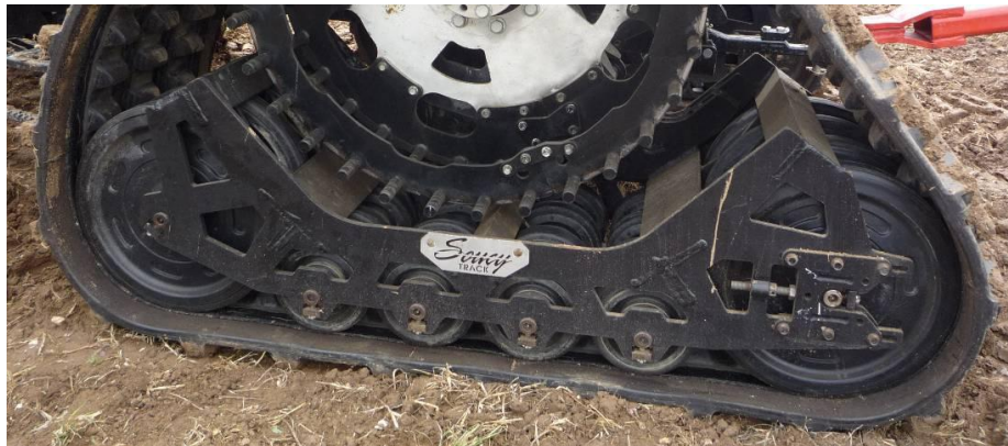
Fig. 5.36. Example of a more favourable design of rubber belt track with many idlers but still with a significant element of the belt unsupported at the extremity of its width.
