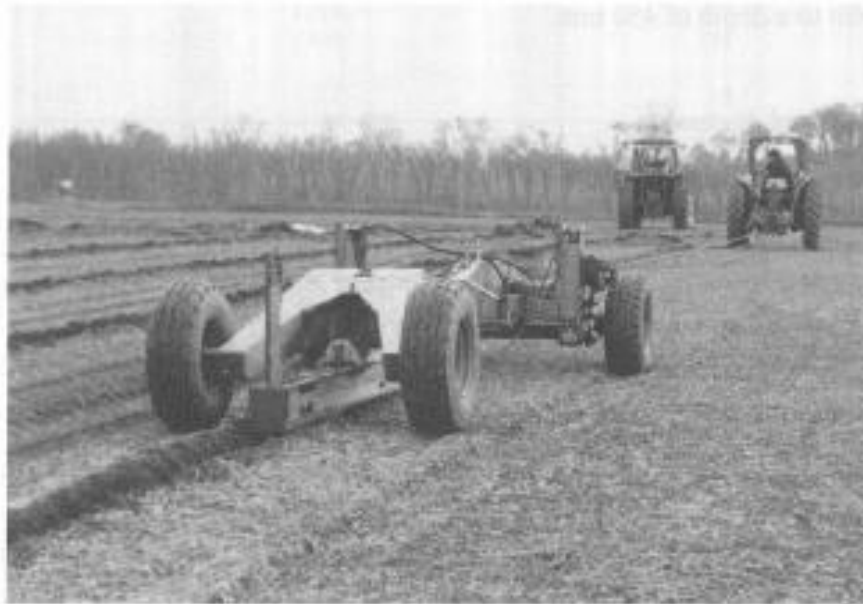
Fig. 1. Winching of the mole plough using a trailed three-point linkage as a stabilizing drawbar.
