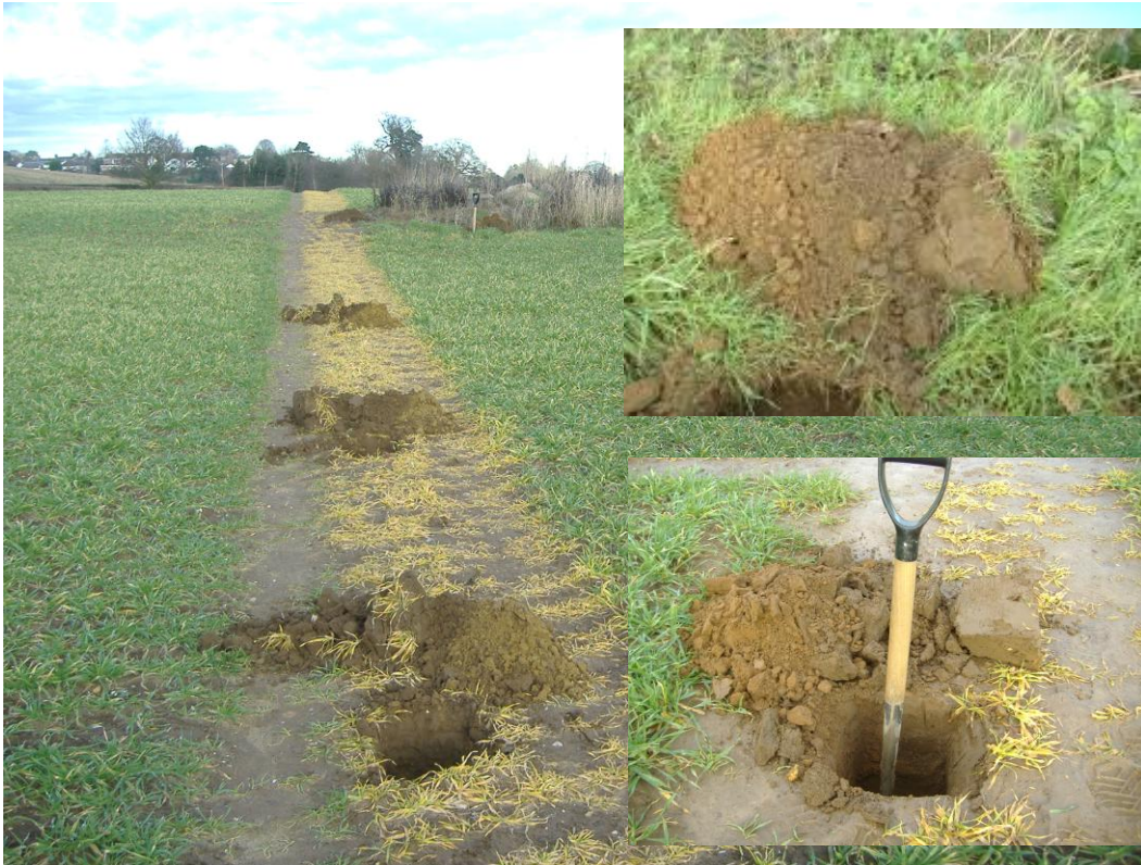
Fig. 4.27. Sandy loam soil showing sampling positions and trafficked (bottom inset) and “non” trafficked soil (top inset)
