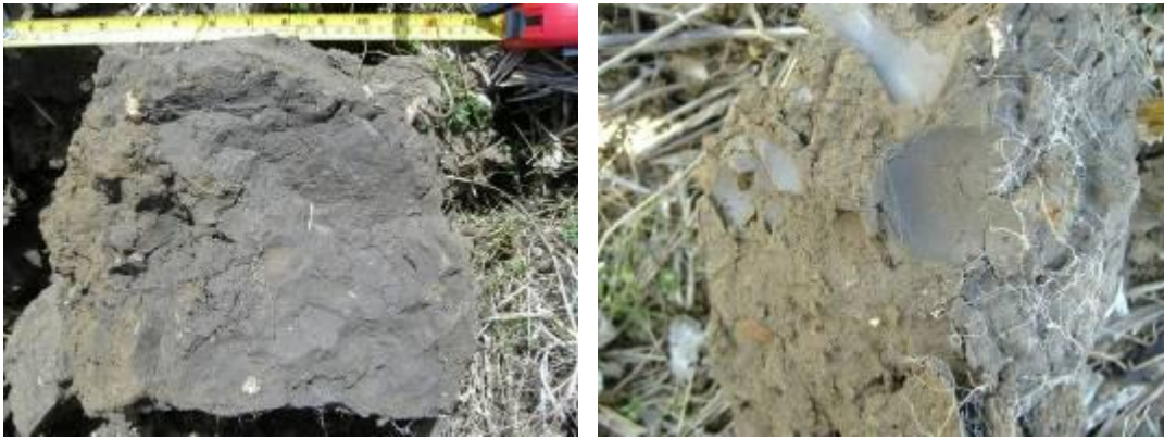
Fig.4.8. Large block of soil removed from 2-year old CTF permanent wheelway (left) and a similar block from a wheelway with a natural fracture (right).
