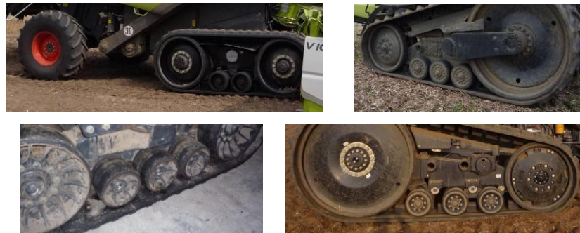
Fig. 5.35. The different track designs involved in the compaction treatments.
