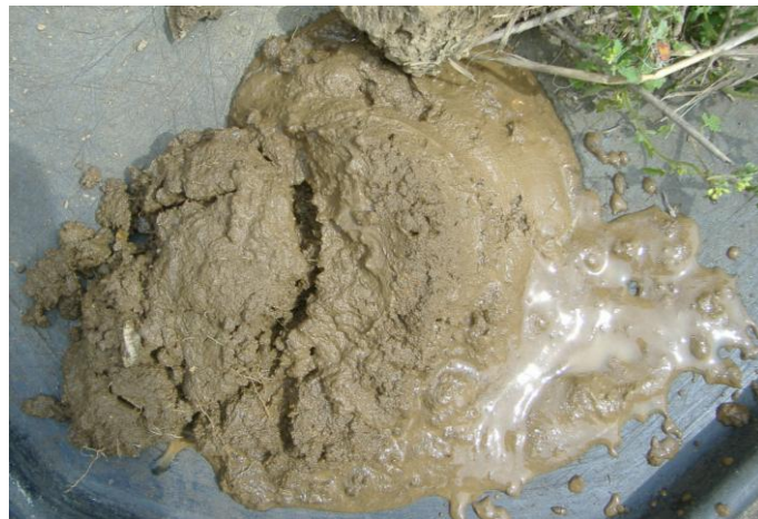
Fig. 4.21. Condition of large aggregate from Normanton Lodge following 90 minutes immersed in water
