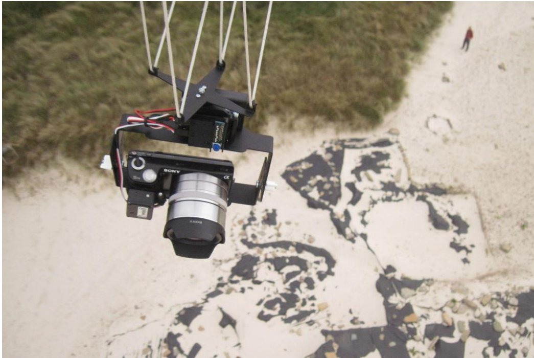
Figure 7.2 - The automatically panning kite aerial photography rig above the site operated by the research-practitioner who is visible in the background. Photograph taken from a secondary rig looking down the kite line.
