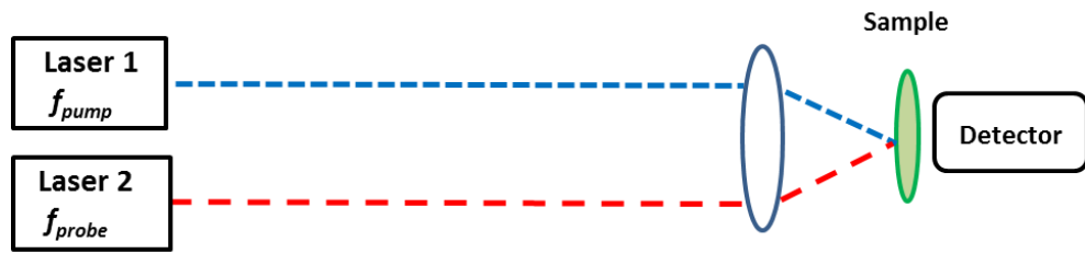
Figure 1-6 – Diagram illustrating the two-laser scanning system of ASOPS, using two slightly detuned repetition rates to investigate the sample.
