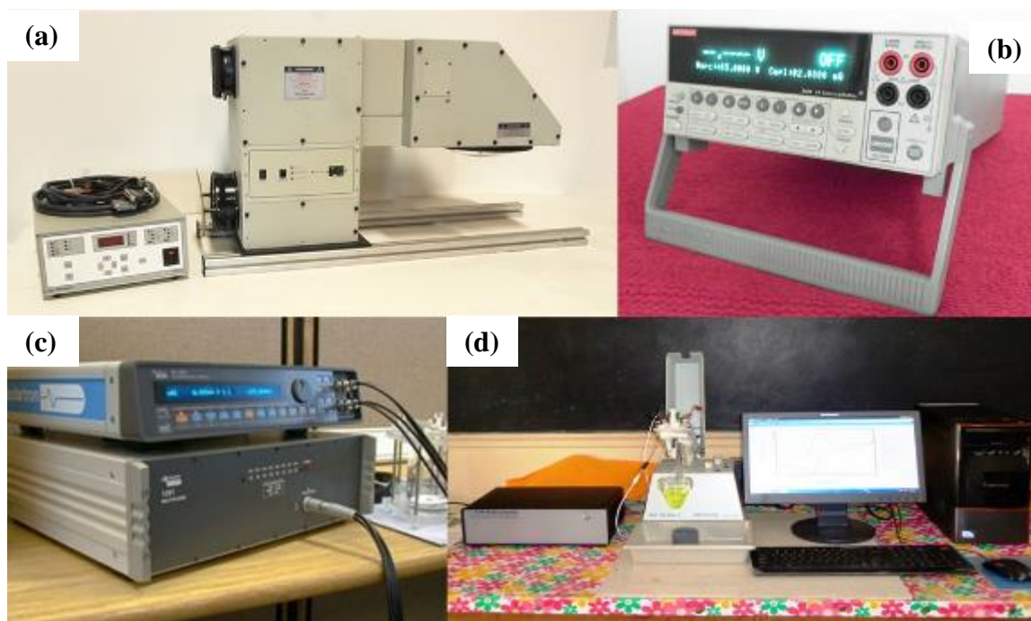
Figure 6.2. Pictures of (a) solar simulator (Oriel); (b) Keithley model 2420 digital source meter; (c) Solartron 1260 Frequency Response Analyzer (upper) in combination with a Solartron 1480 Potentiostat (lower); (d) CHI660d electrochemical workstation.
