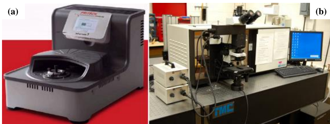
Figure 7.2. (a) PULVERISETTE-7 planetary ball milling machine and (b) HR800 Raman spectrometer.
