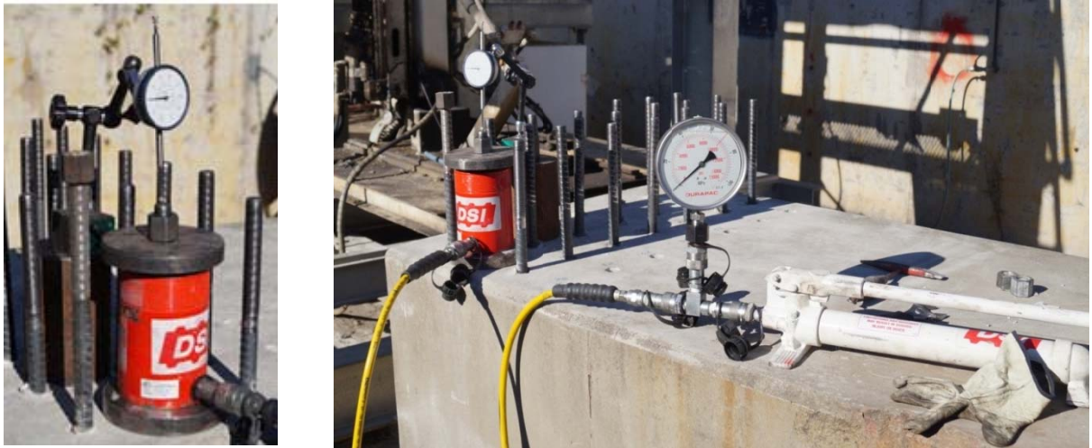
Figures 9a and 9b: Pull test experimental setup – 300 mm embedment, 28 mm and 30 mm hole diameters
