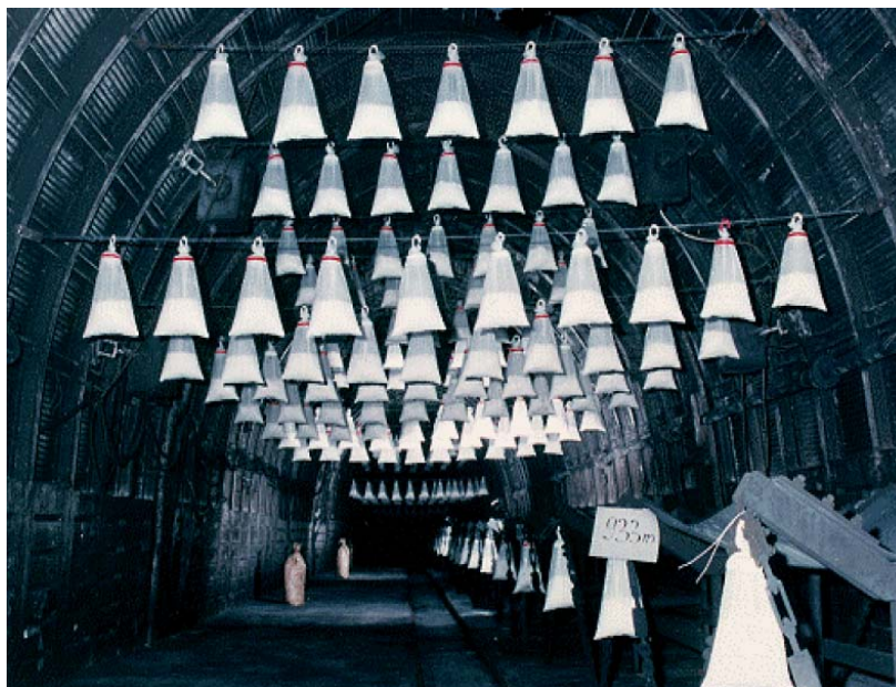
Figure 5: Bagged stone dust barrier (Belle and Du Plessis, 1999)
