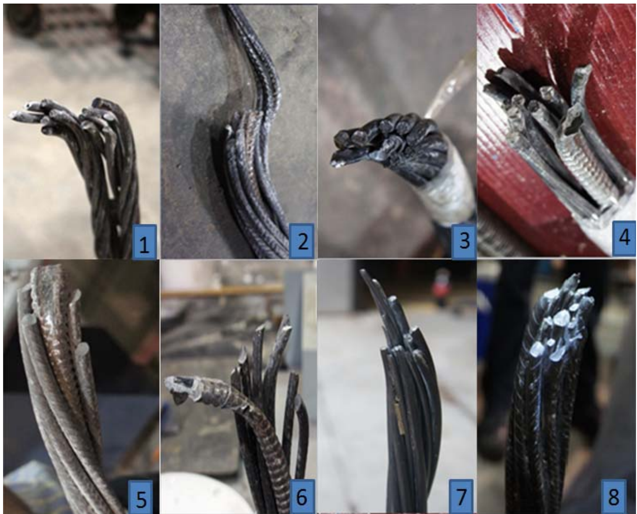
Figure 14: strands snapped of the tested cables
