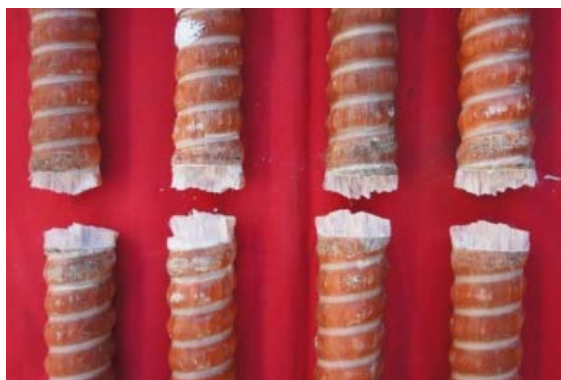
Figure 5: Single sheared failed 22 mm diameter dowels
