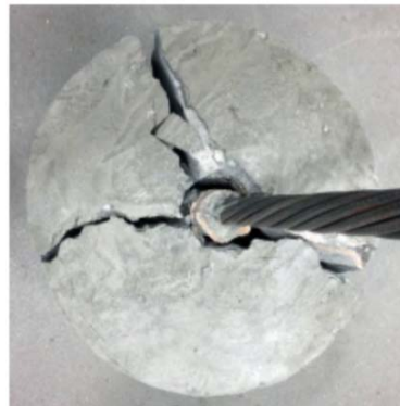
Figure 12: Typical failure mode of test samples with two or three fractures
