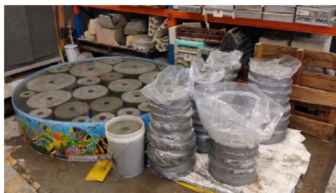
Figure 7: Test samples fully submerged in water for curing
