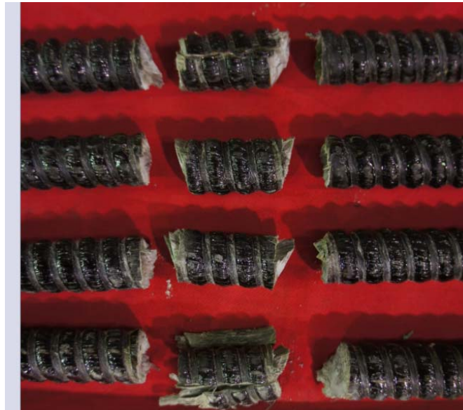
Figure 8: failure pattern of dowels in guillotine
