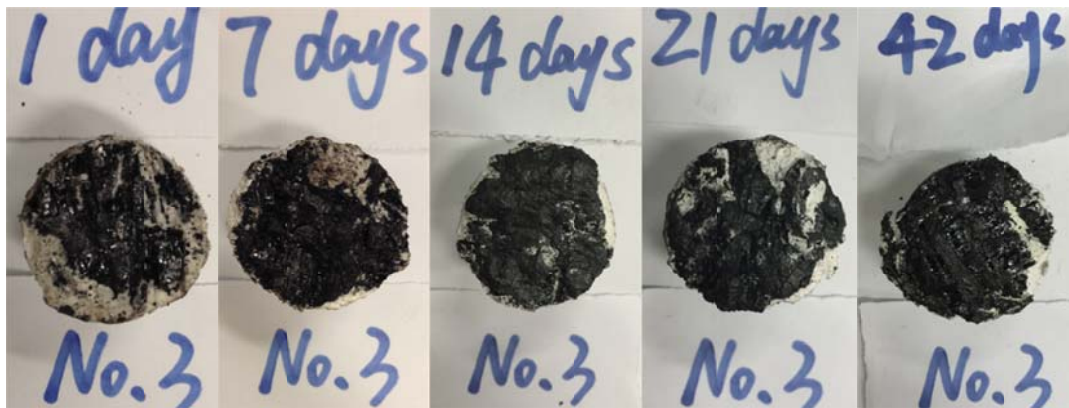
Figure 8: Typical view of failure surface with different curing time
