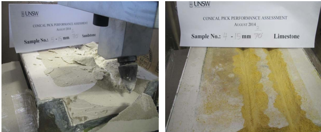
Figure 5: Cutting with a pick tip angle of 70° at 15mm depth of cut in Gosford Sandstone (left) and Gambier Limestone (right)
