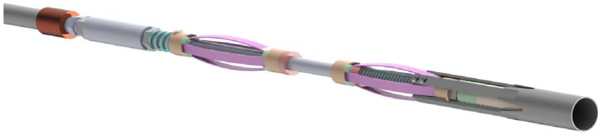
Figure 9: Prototype water jet cable bolt drill currently in development by CRCMining
