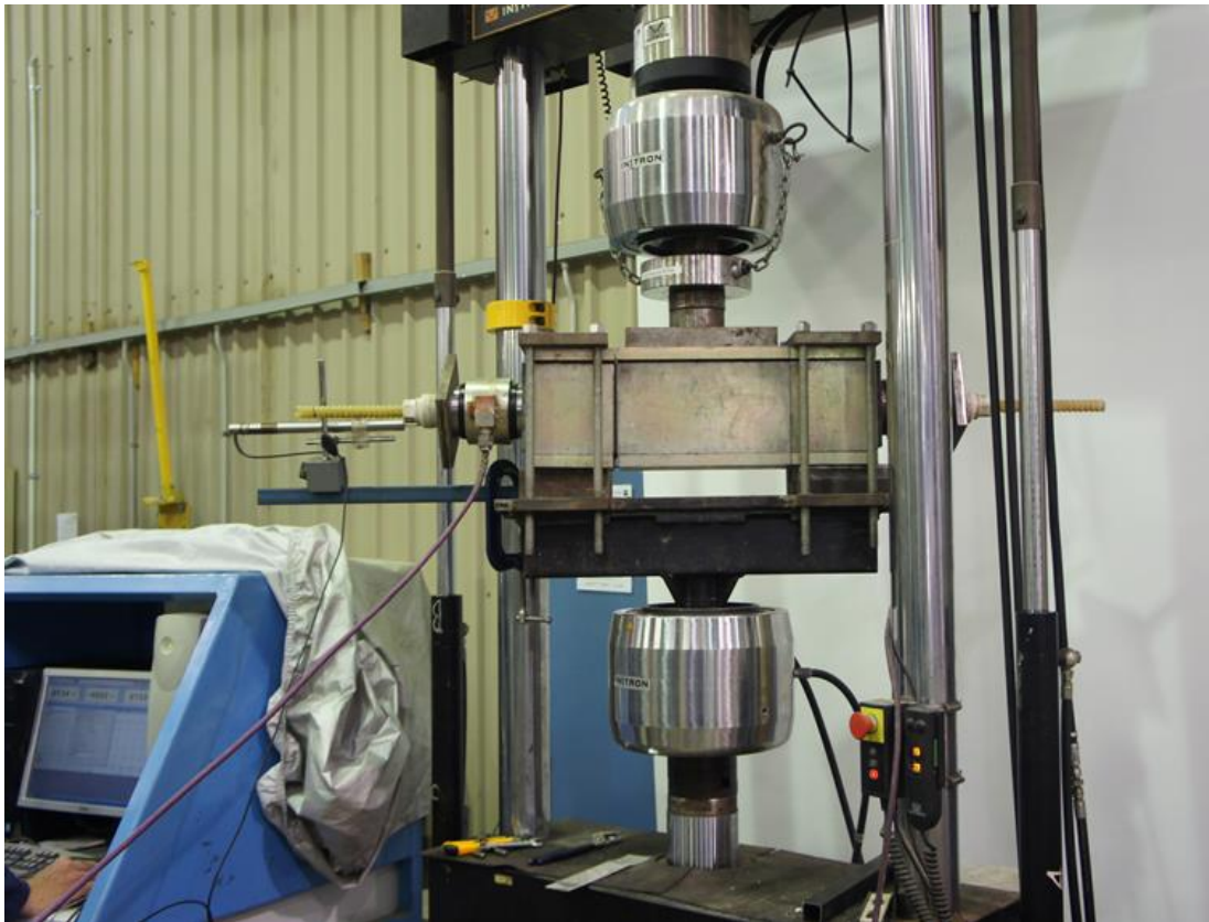
Figure 9: An assemble FG dowel with load cells for double shear testing in 50 t Instron testing machine
