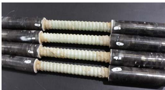
(a) Intact 500 mm long dowels with short end encapsulation
