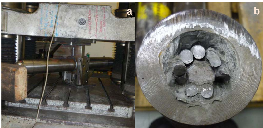
Figure 6: Shear test and a view of the sheared sample. Note the interaction between the strands and the steel tube
