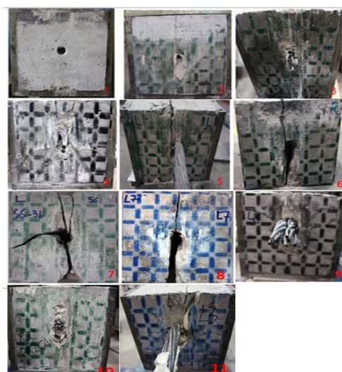
Figure 9: Concrete block surfaces after shearing
