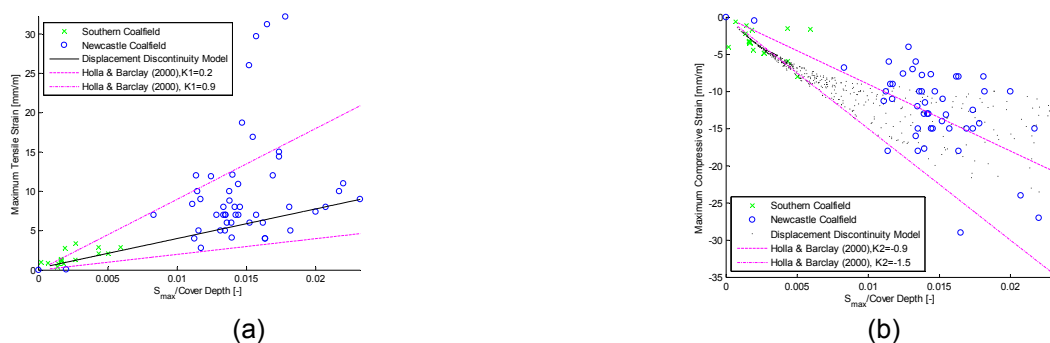
Figure 4: Relationships between maximum tensile strain (a) and compressive strain (b) to maximum subsidence in terms of cover depth of longwall panel. Data sources: Ditton and Frith (2003) and collected field data
