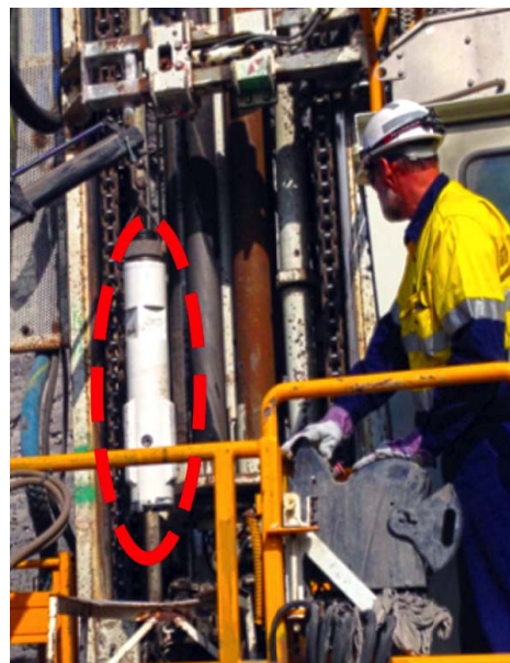
Figure 1: Schematic of water separator sub in a blasthole (NIOSH, 2012) (left) and, installation of the sub (right)
