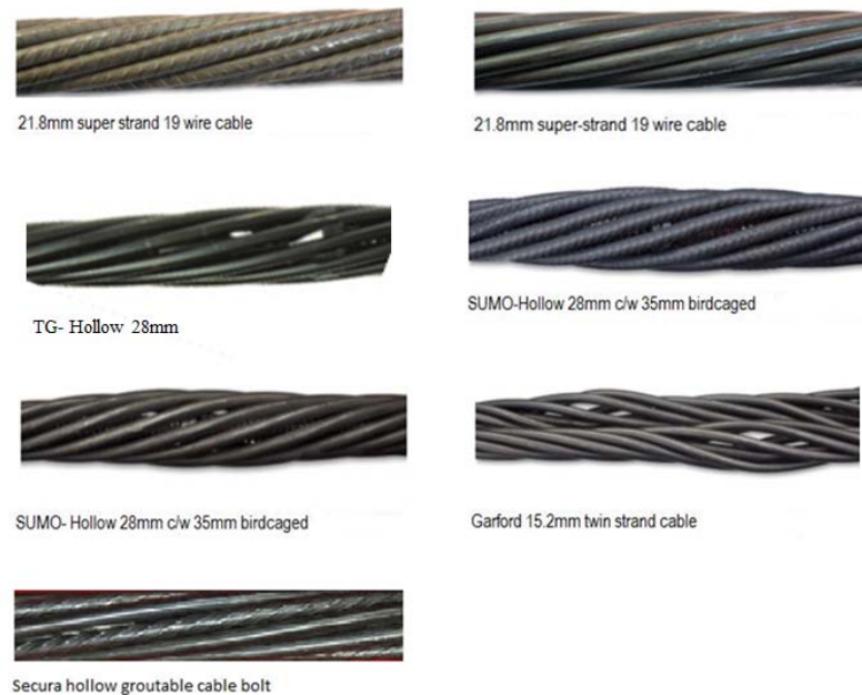
Figure 7: Cable bolts used for double shearing test purpose
