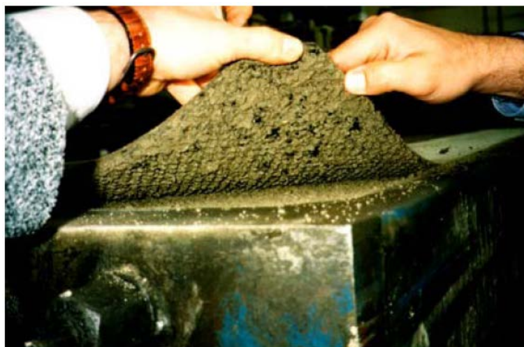
Figure 2: Gluing System using adhesion (courtesy: DelkorRail)
