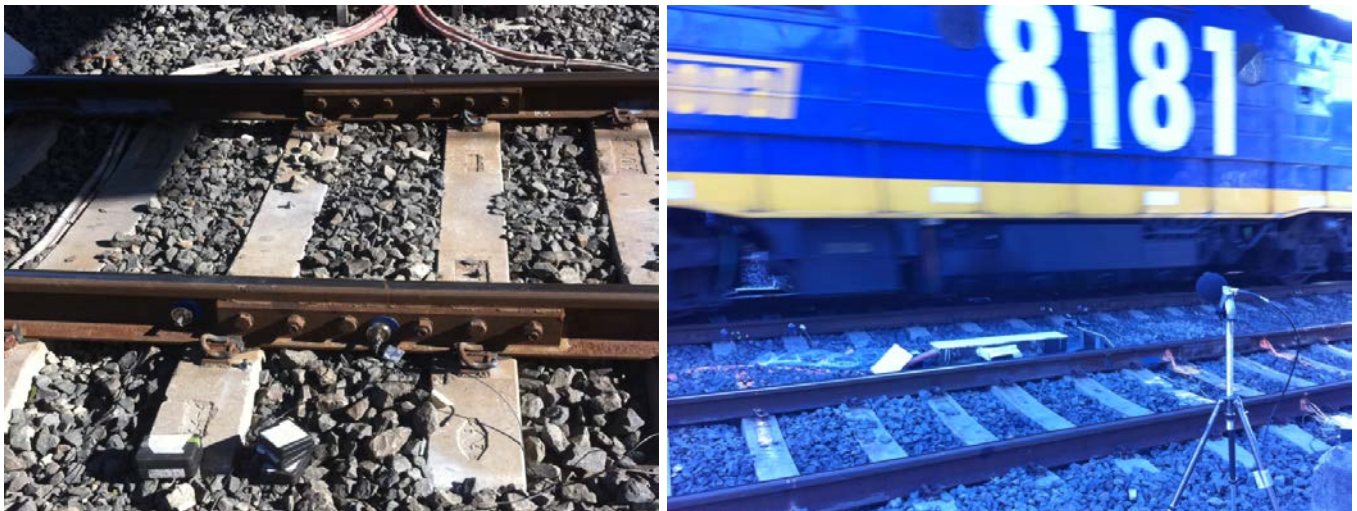
Figure 16: Instrumentations at the test site (accelerometers, deflectometers, speed radars, microphone array, high-speed camera)
