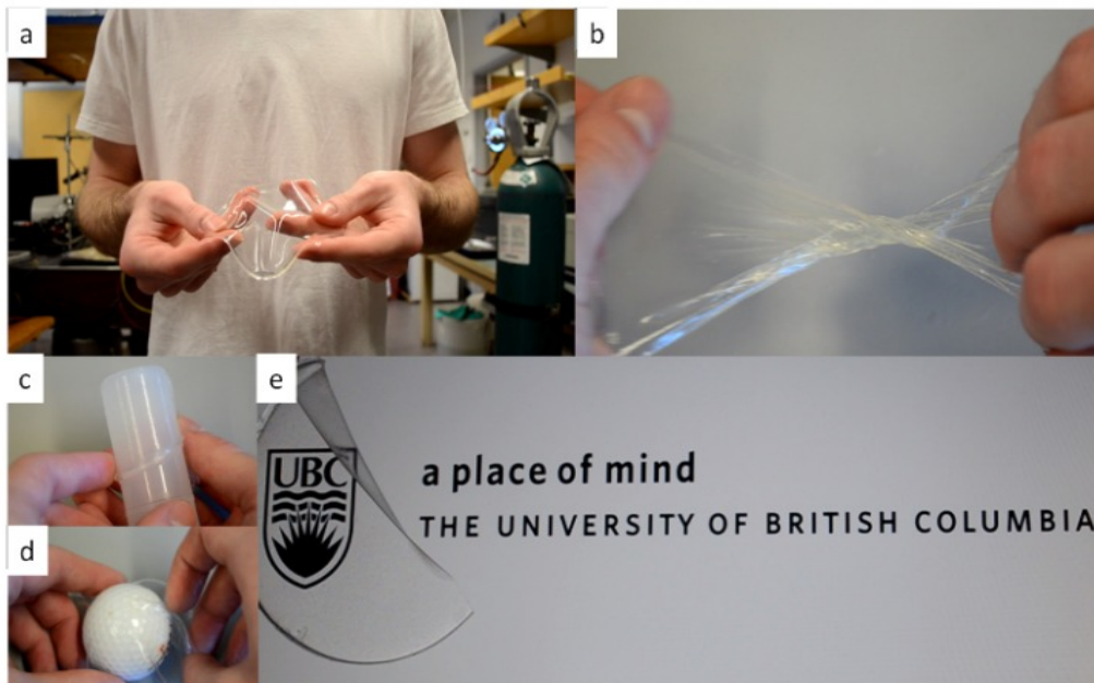
Figure 1: Piezoionic material showing conformity, transparency and mechanical strength
