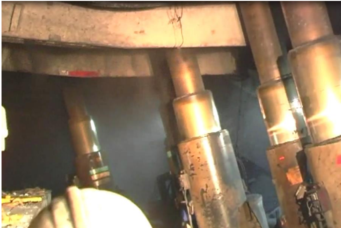
Figure 3.10 Dust from a Chock as it is Set to the Roof
