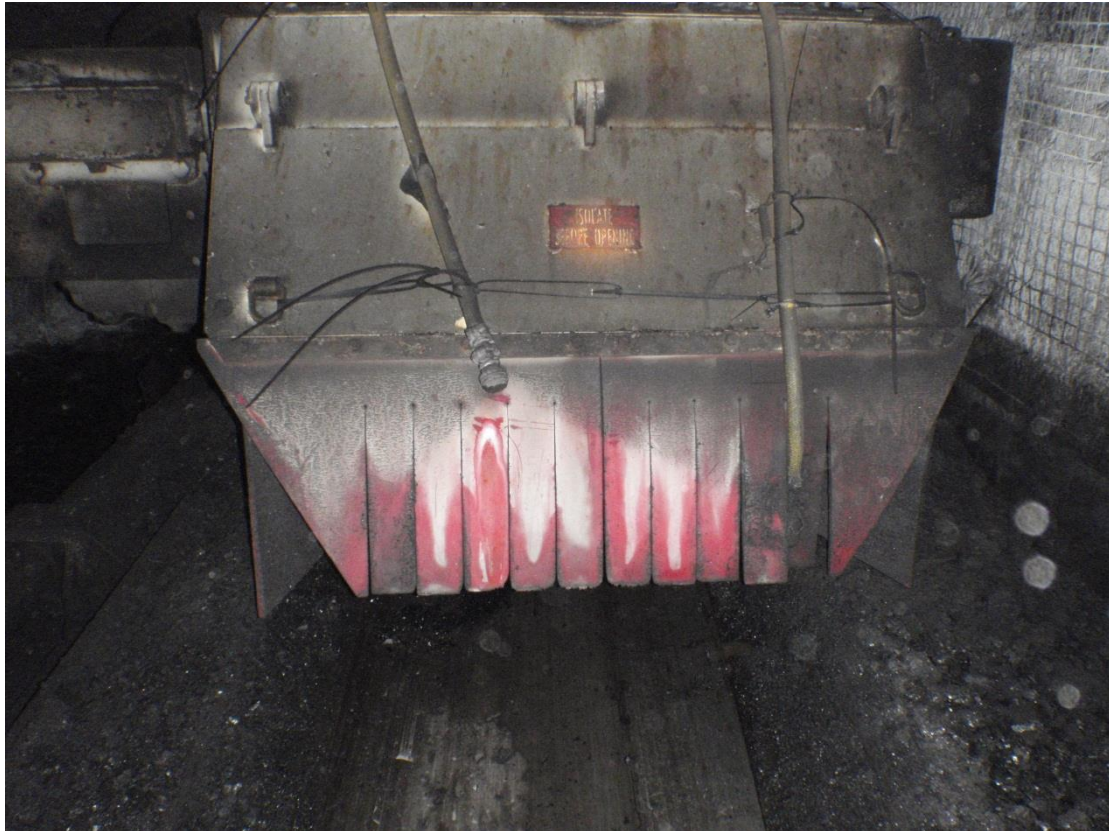
Figure 3.5 Typical BSL Discharge
