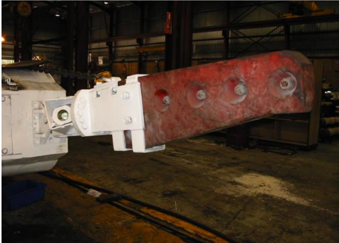
Figure 4.11 Typical Shearer Clearer Setup
