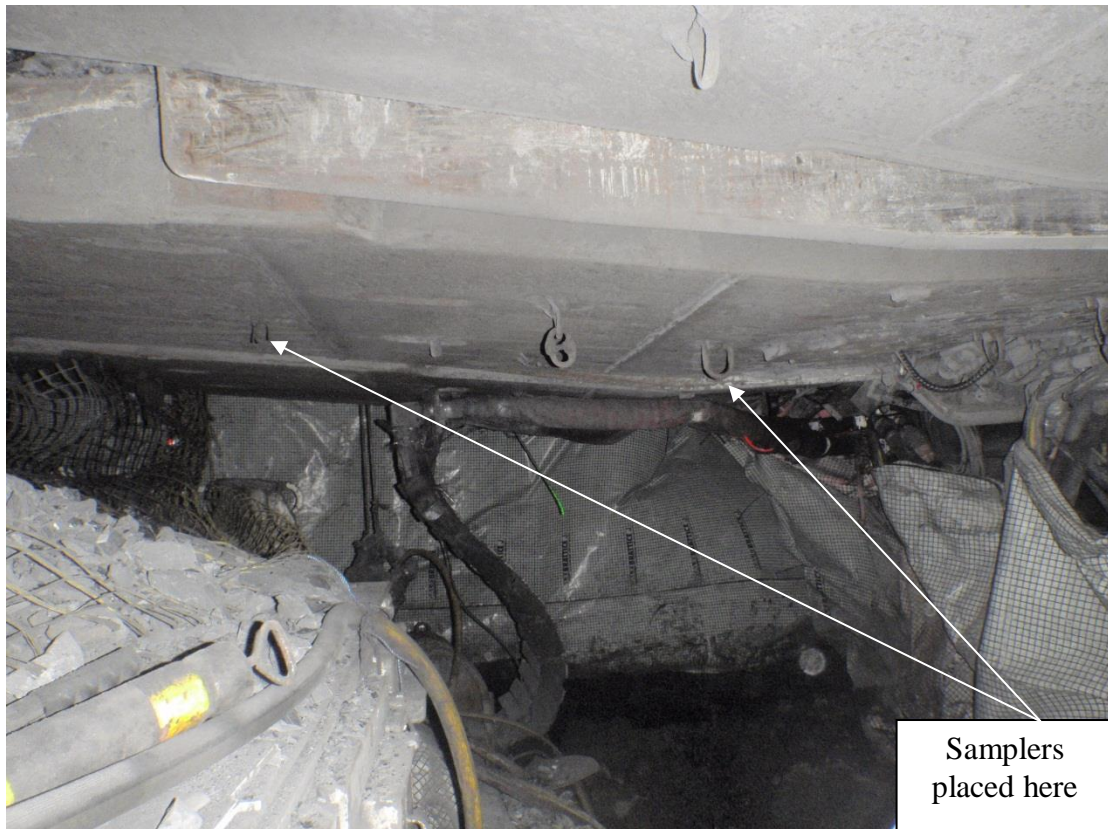
Figure 7.48 Mine C Pump and Head Location for Crusher Dust on Chock #5
