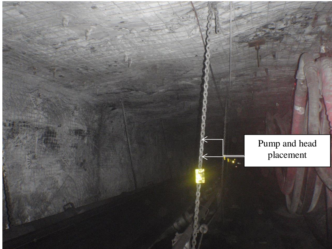
Figure 6.4 Pump and Head Placement in Belt Road
