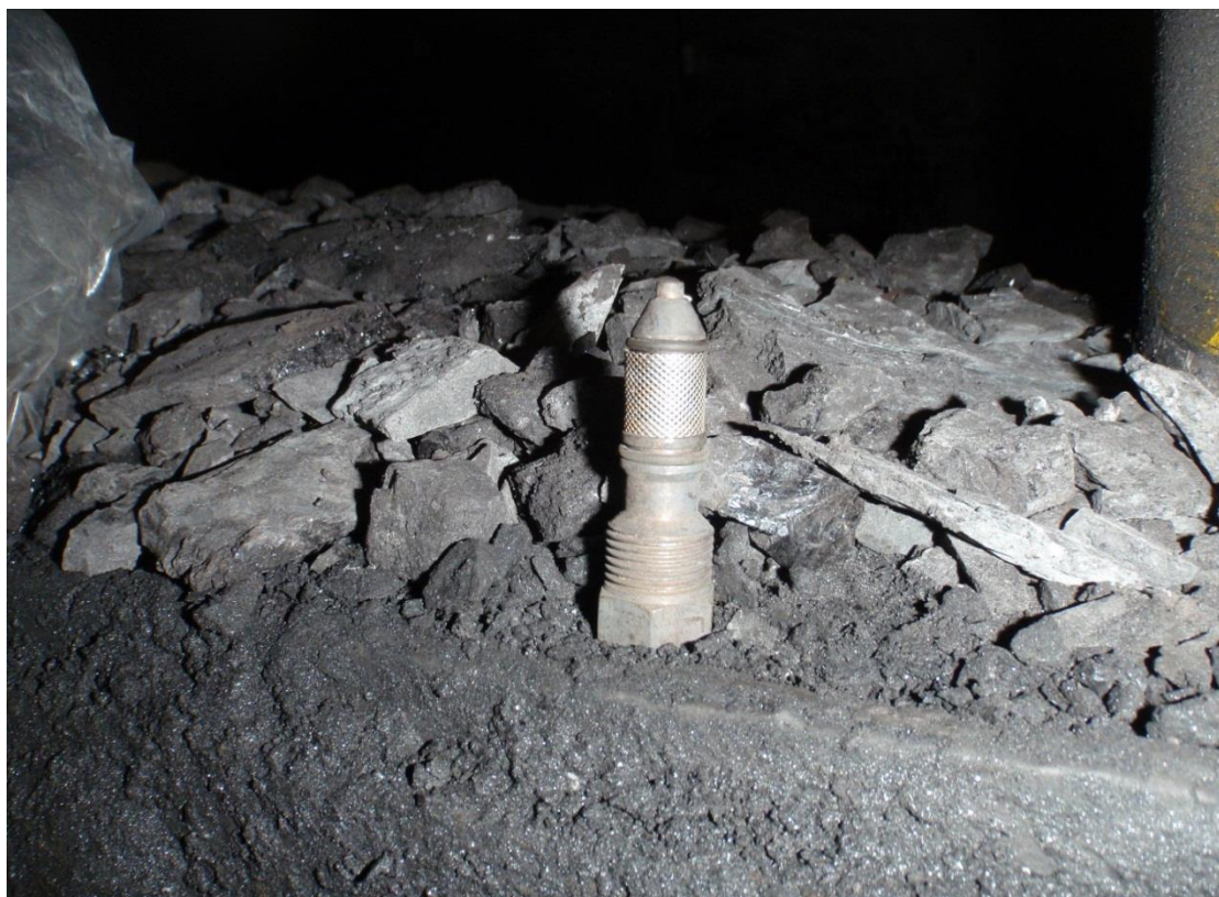
Figure 4.9 Typical Spray Insert in Drum Sprays
