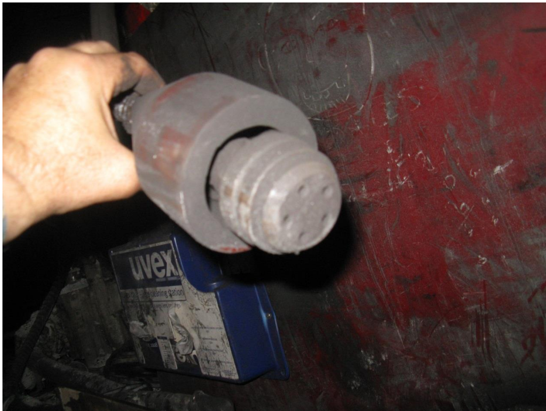
Figure 7.37 Mine B Code 96 Fitted to Dropper Spray
