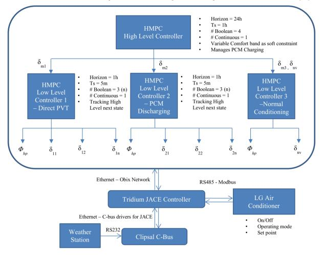
Fig. 4. Schematic of the control system architecture developed in the present project.
