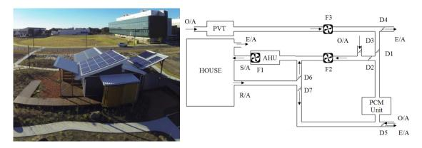
Fig. 1. (a) The Team UOW Solar Decathlon house; (b) HVAC system schematic (where S/A, O/A and E/A are the supply, outside and exhaust air, respectively, and Fn and Dn represent fans and dampers).
