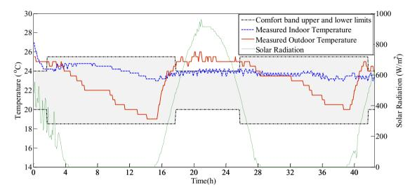
Fig. 6. Temperatures and solar radiation of HMPC experimental results for the Team UOW Solar Decathlon house in Wollongong, Australia,  $(t = 0 \text{ is equivalent to } 3:20 \text{ pm } 16^{\text{th}} \text{ February } 2015).$
