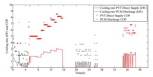
Fig. 8. Instantaneous cooling rates and COP of case study system corresponding to Fig. 6.
