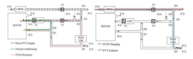
Fig. 3. Schematic of: (a) HVAC system conditioning operating modes; and (b) HVAC system PVT modes.
