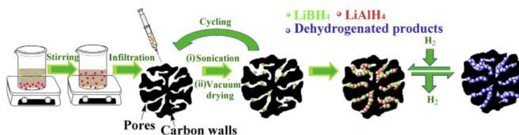
Figure 5. 1 Schematic diagram of the preparation process for nanoconfined 2\text{LiBH}_4\text{-LiAlH}_4 composites
