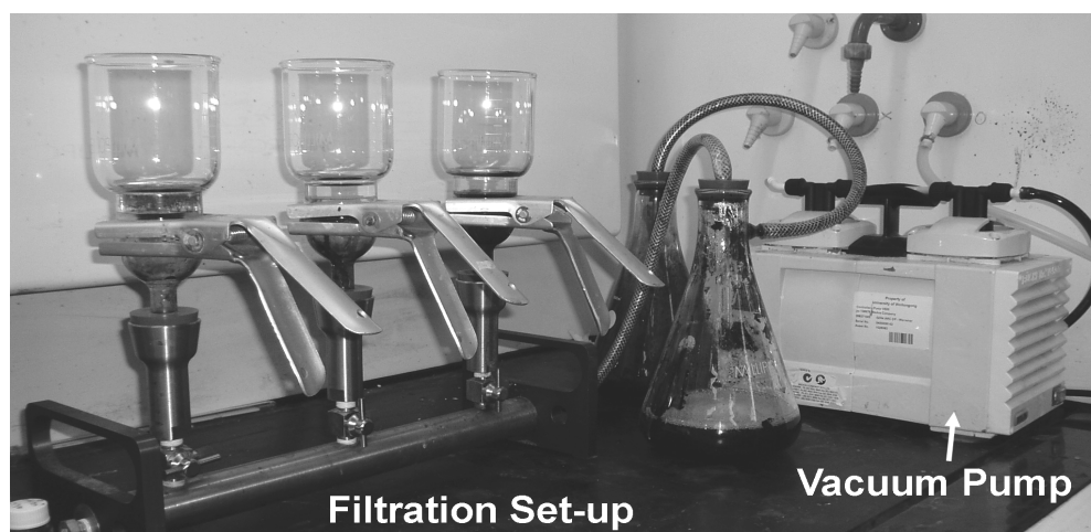
Fig. 3.2 The filtration setup for the fabrication of CNT film.
