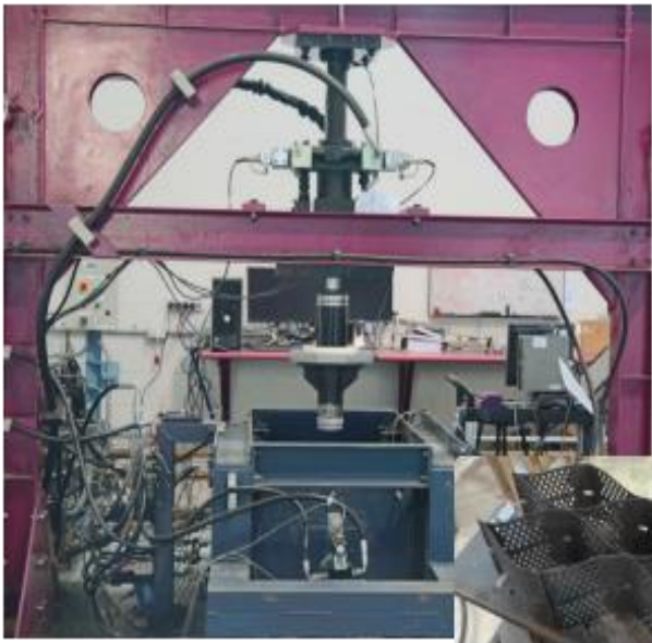
Fig. 4 Process Simulation Prismoïdal Triaxial Apparatus (PSPTA) designed and built at University of Wollongong.
