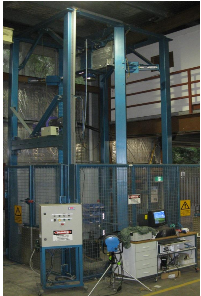
Fig. 14 Drop weight impact testing equipment.
