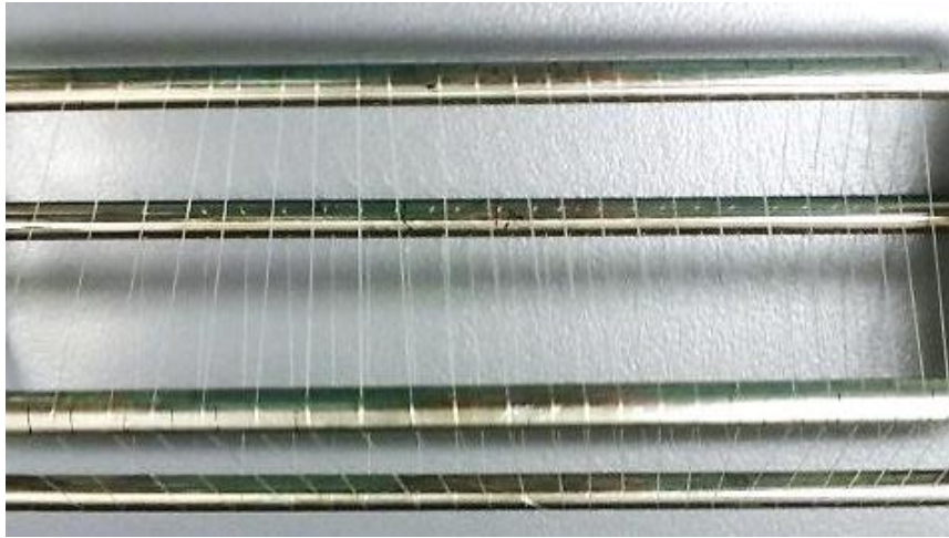
Figure 3 The capability of producing unlimited length of coaxial Chit-Alg (1) fibres as shown onto a collector
