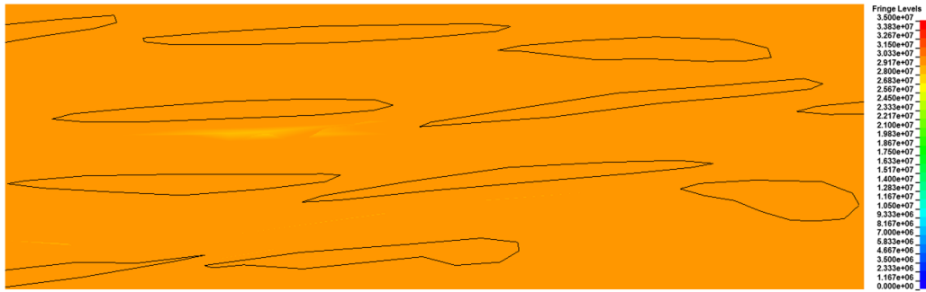
Figure 5.53: Stress contour (indicated by fringe levels in Pa) in the dendritic structures at maximum deformation under rolls 60% reduction (Model 4).
