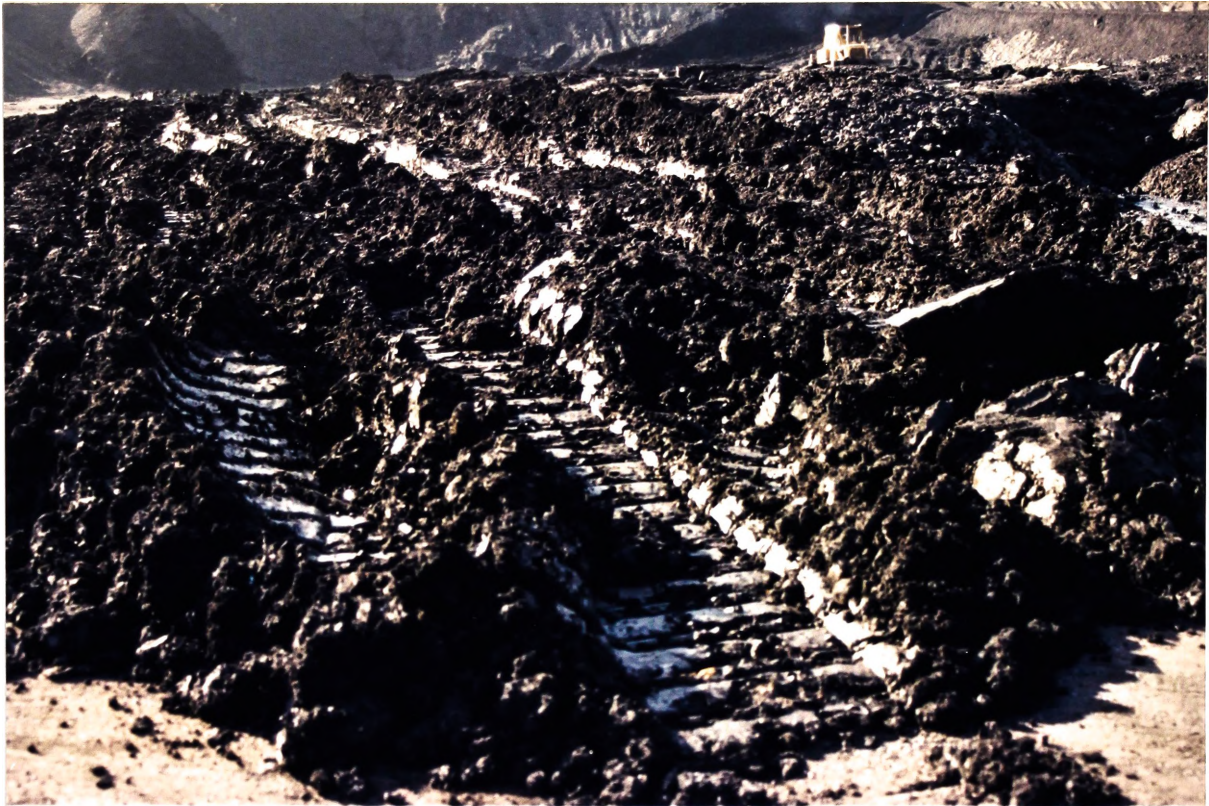
Figure 2.9: Slimes Dumped Separately in Impoundment
