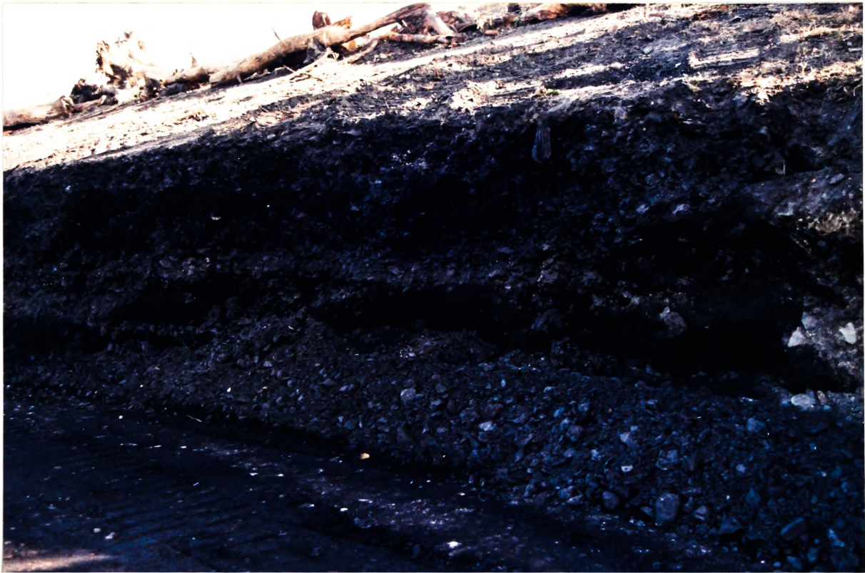
Figure 2.8: Cross-section Through Layered Sequence of Reject Material
