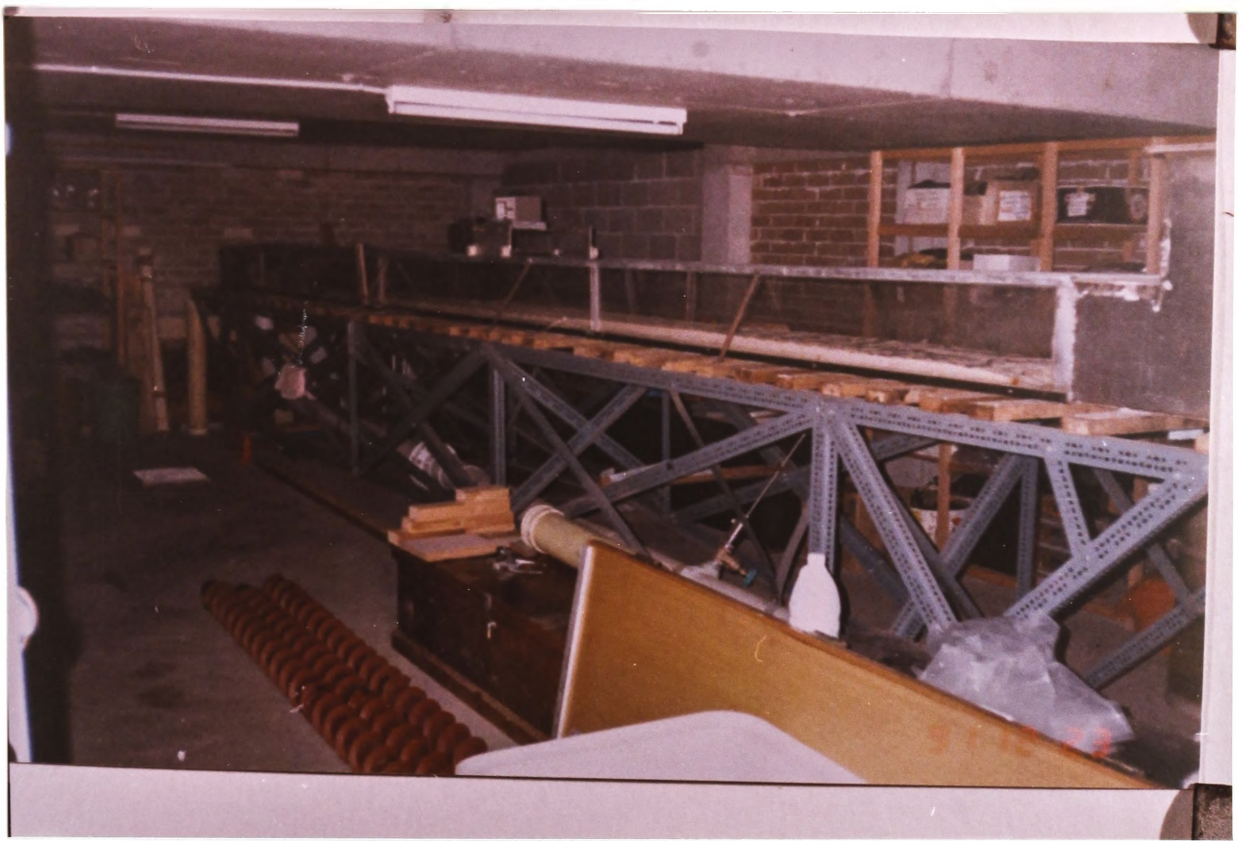
Plate 3.1 General view of the recirculating flume showing the inlet section (right). The channel is 0.45 m wide and 10 m in length.
