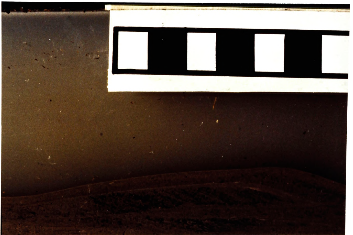
Plate 4.4 Small low amplitude ripple encased by a larger, compacted ripple (Run 17). Aggregates are clearly evident in the smaller ripple but not in the larger ripple.
