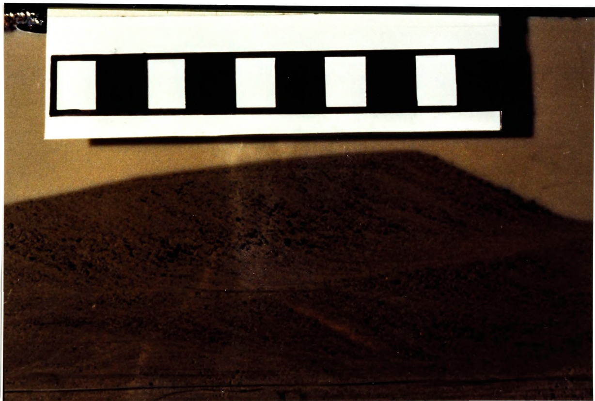
Plate 4.1 (Top) Asymmetrical ripples showing well-developed foreset laminae (Run #23). Scale divisions 1 cm long.
