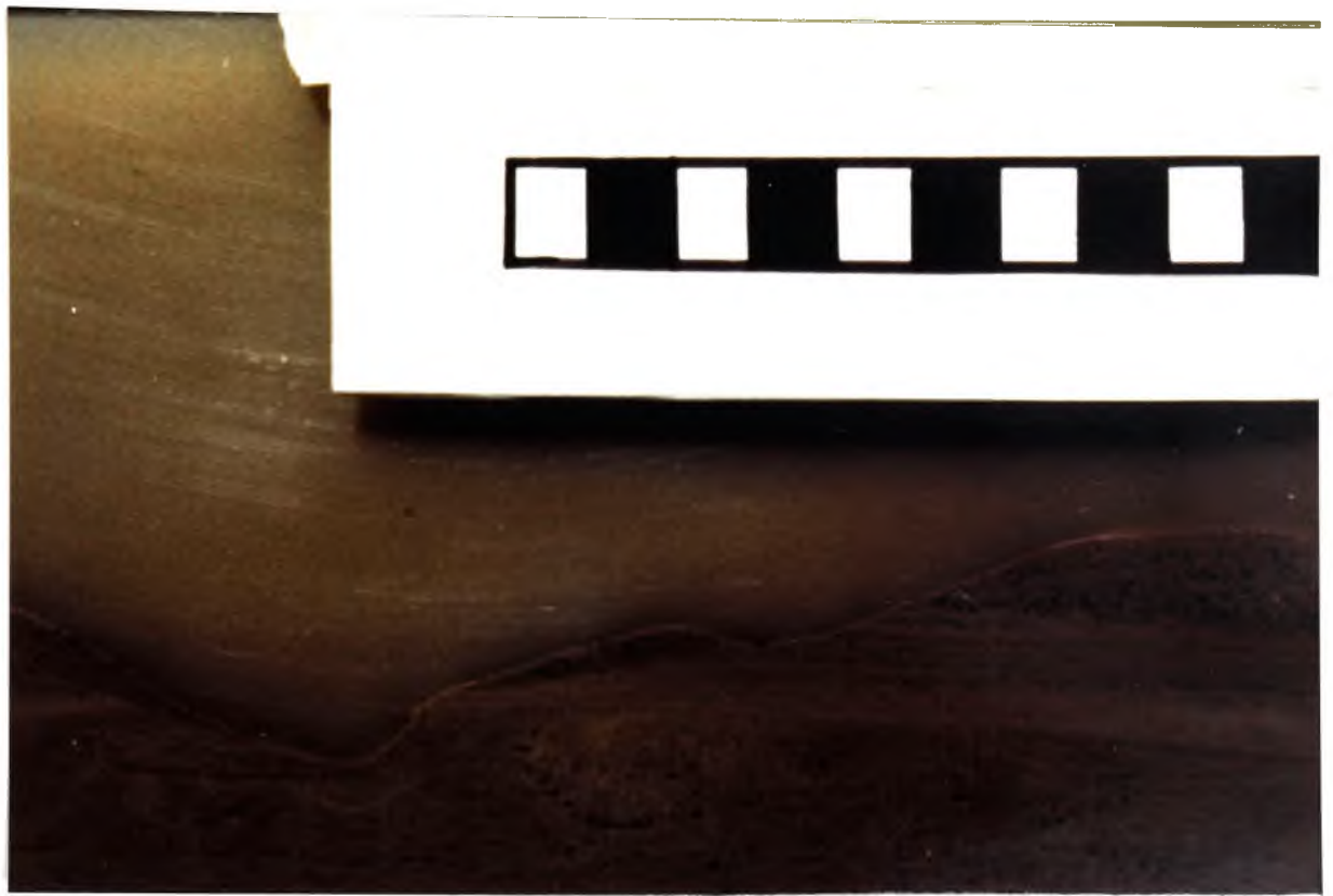
Plate 4.3 Deep scourhole located behind a small climbing ripple (centre) which trails a larger ripple (Run 3). Flow is from left. Scale: 1 unit = 1 cm.
