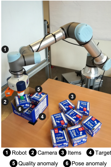
Fig. 5. The experimental setup for evaluating the introduced deep PGP framework.
