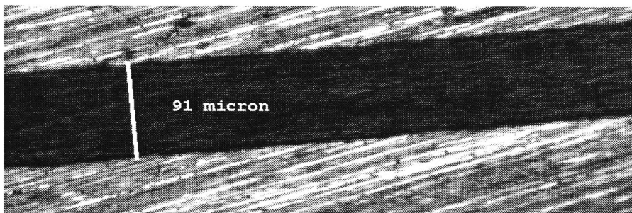
Figure 3.11. Interface between insulation composite D and HTS tape in Pancake coil 12.
