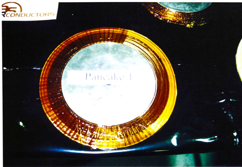
Figure 3.6. Pancake 1 after curing
