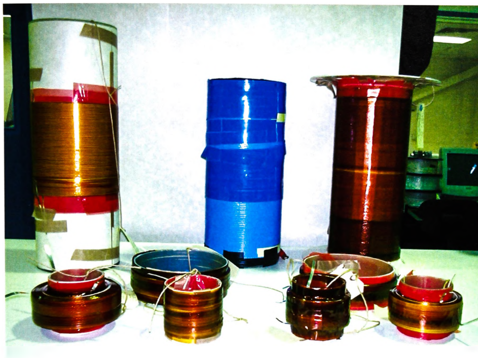
Figure 3.18. A selection of manufactured solenoid coils.
