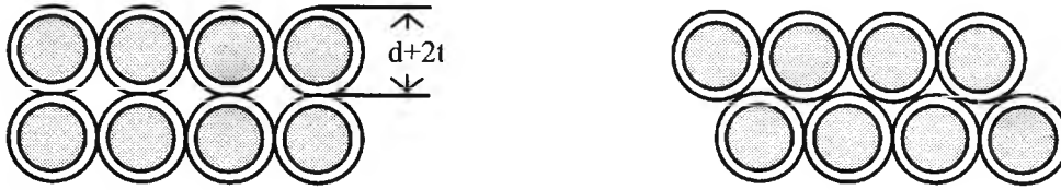
Figure 3.1 Diagram of the different structures possible with round wires
