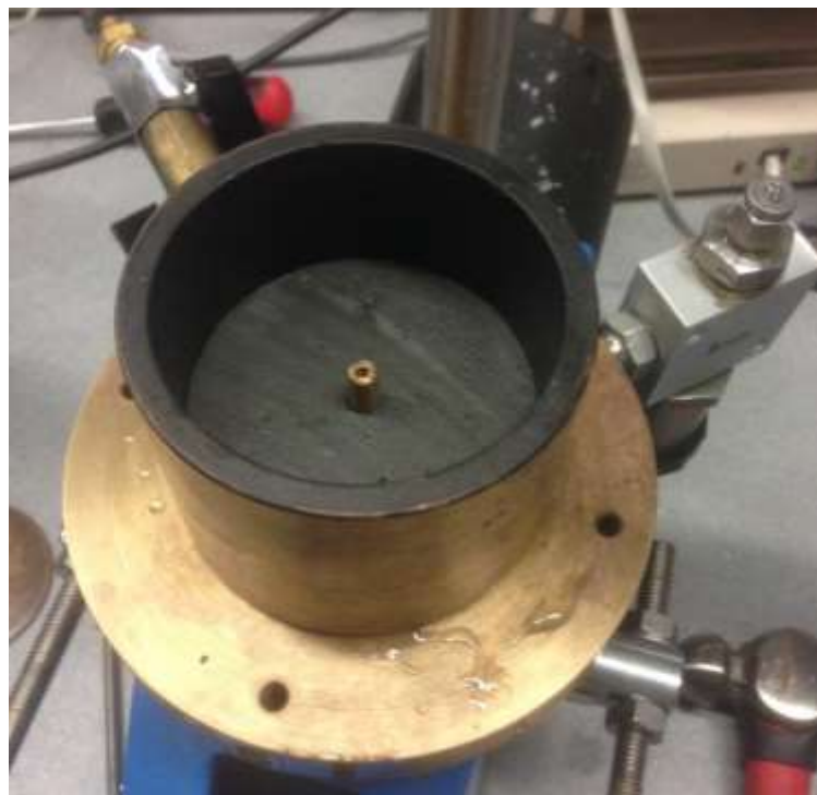
Figure 5.12 : Drain installed undisturbed sample before starting consolidation.
