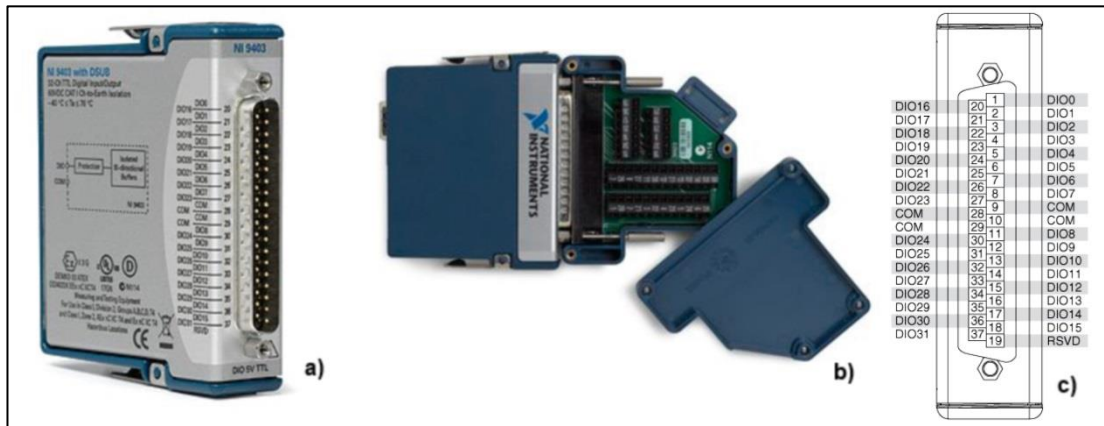
Figure 4.3. a) NI 9403 module. b) NI 9403 module with NI 9923 terminal block attached. c) NI 9403 module terminal assignments [102, 103].
