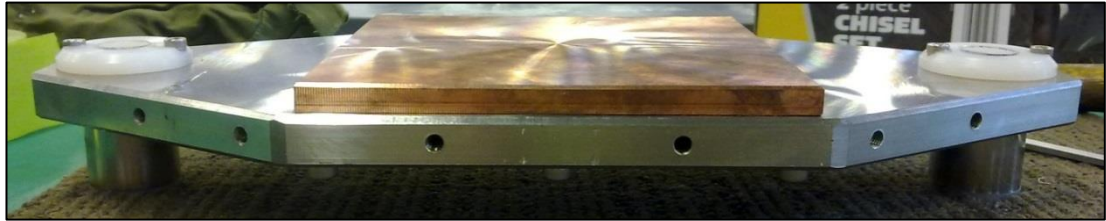
Figure 3.15. A view of a fully assembled cooler.
