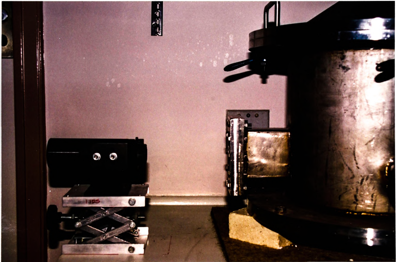
Figure 44, optical pyrometer sighted into custom built oven.
