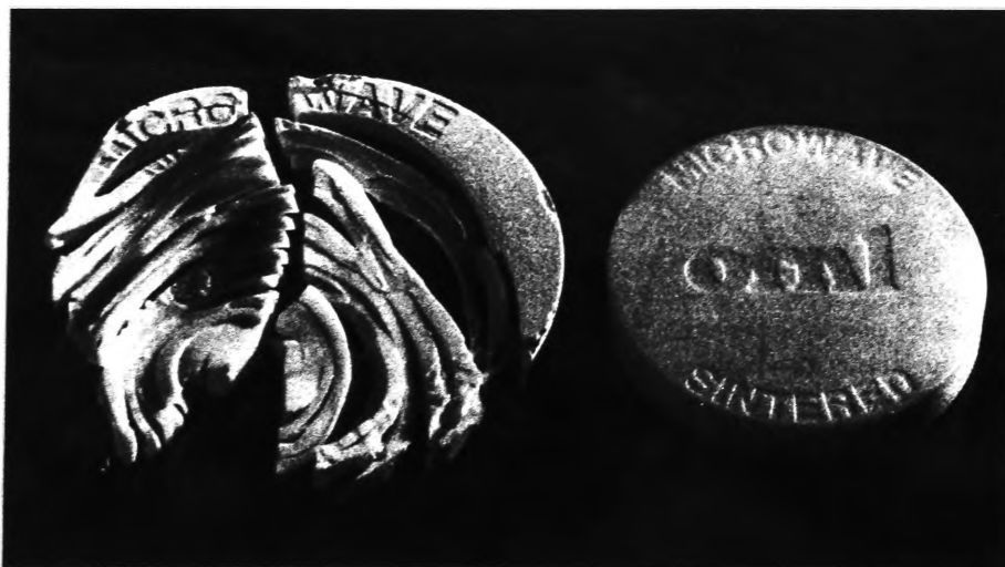
Figure 23, Y-PSZ sintered at 2.45GHz and 28GHz. From Janney et al. 11
