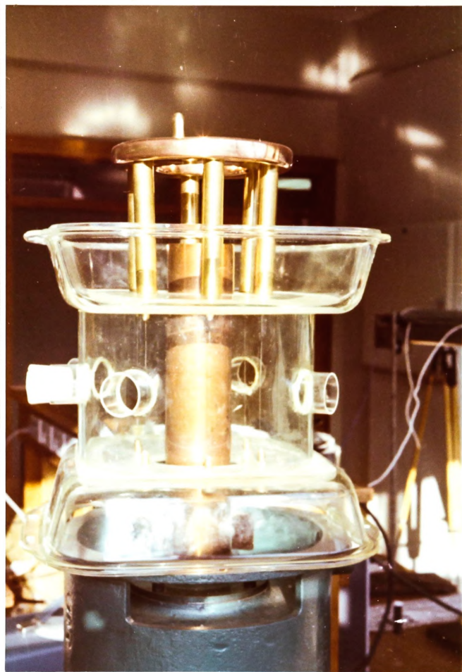
(B) Pyrex glass used throughout. Excellent corona characteristics at all temperatures.
