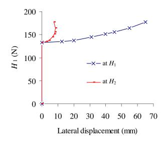
Fig. 14 Lateral displacements of two-span continuous beam [41]
