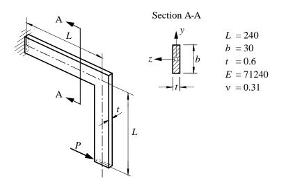
Fig. 1 Cantilevered right-angle frame subject to flexural-torsional buckling [23]
