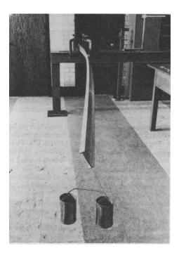
Fig. 10 Lateral buckling of a doubly-symmetric I-section cantilever [35]
