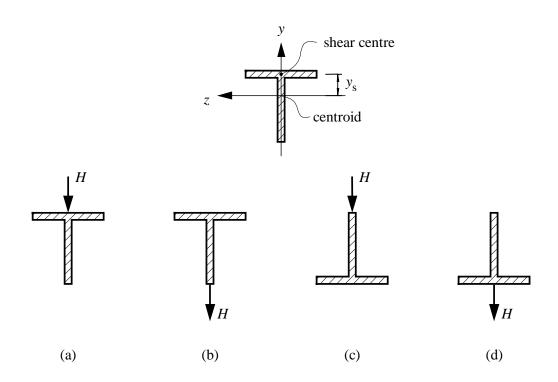
Fig. 11 Tee cantilevers loaded in various ways [36]
