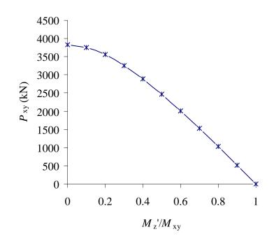
Fig. 9 Buckling loads of simply supported doubly-symmetric I-section beam-columns
