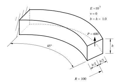
Fig. 17 Curved cantilever [53]
