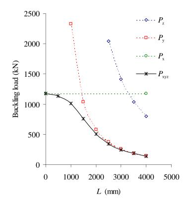
Fig. 6 Buckling loads of simply supported unequal angle columns
