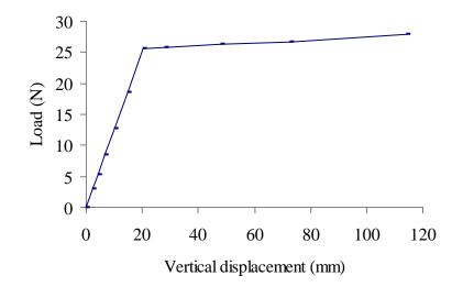
Fig. 12 Load-deflection graph of cantilever [35]
