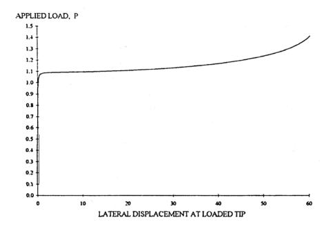
Fig. 2 Detecting "bifurcation" buckling by means of perturbation [20]
