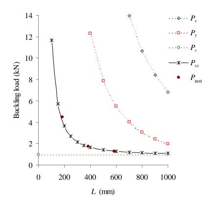
Fig. 8 Buckling loads of simply supported lipped equal angle columns
