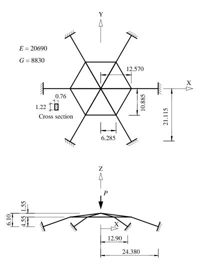
Fig. 3 Space dome subject to flexural-torsional buckling [25]
