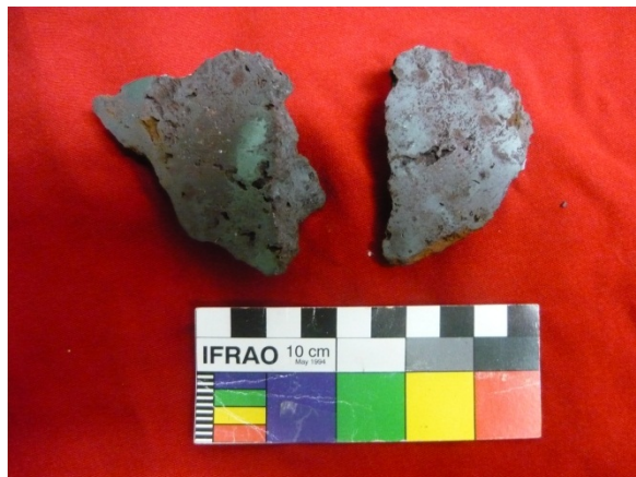
Fig. 4.9 : Picture of hematite block, cut in half prior to experimentation
