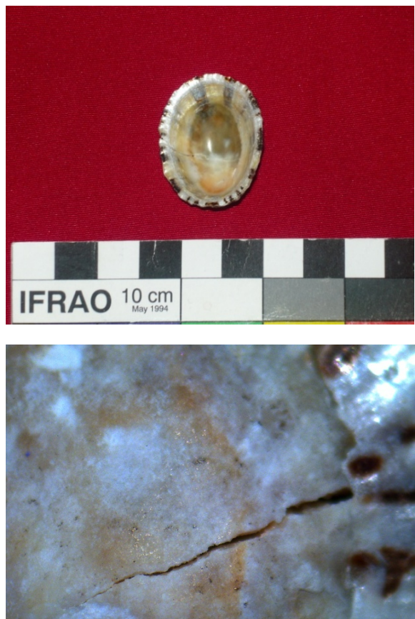
Fig. 5.11 : Results of INSTRON controlled fracture experiment of C. solida with pictured breakage patterns
