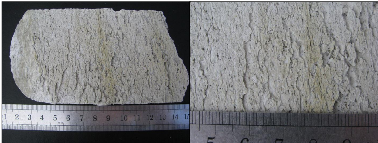
Figure 22: Sample C03 (TYHD004; 142.10 m) section offcut.
