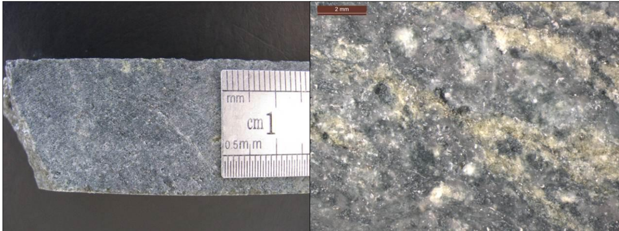
Figure 24: Sample C08 (TYHD004; 349.5 m) section offcut.
