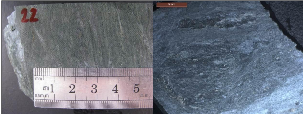
Figure 28: Sample C22 (TYHD003; 279.00 m) section offcut.
