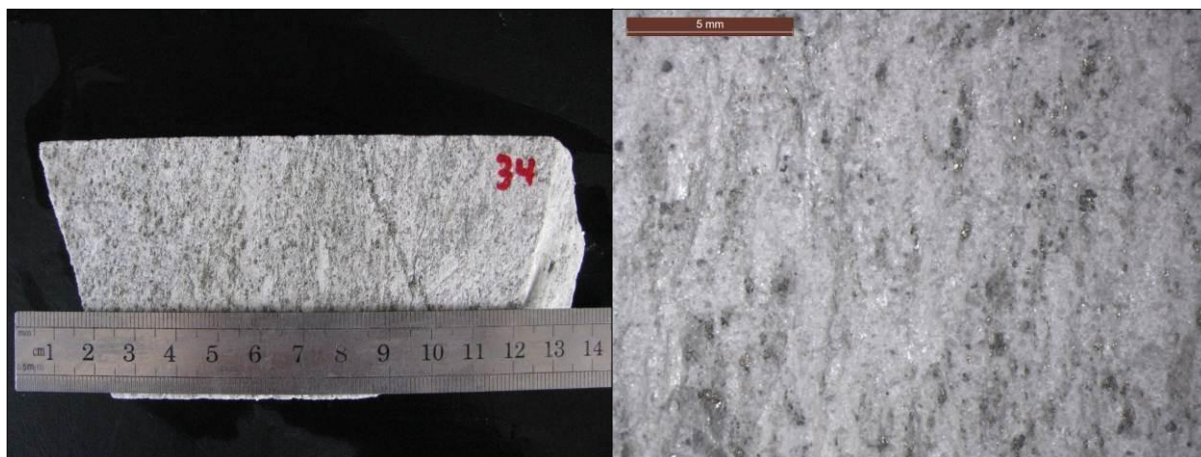
Figure 33: Sample C34 (TYHD005; 60.0 m) section offcut.
