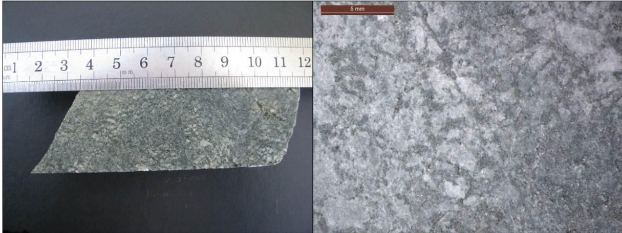
Figure 34: Sample C35 (TYHD005; 359.5 m) section offcut.
