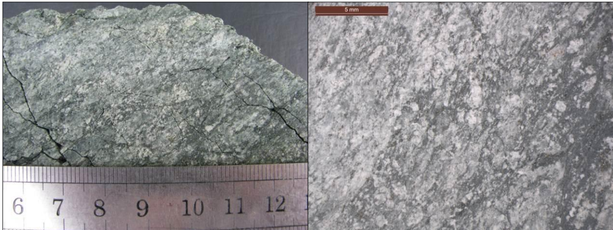
Figure 23: Sample C04 (TYHD004; 208.95 m) section offcut.
