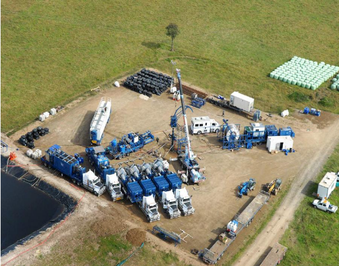
Figure 41 Typical CSG hydraulic fracturing operation in Gloucester, NSW (Source: AGL Energy Ltd)
