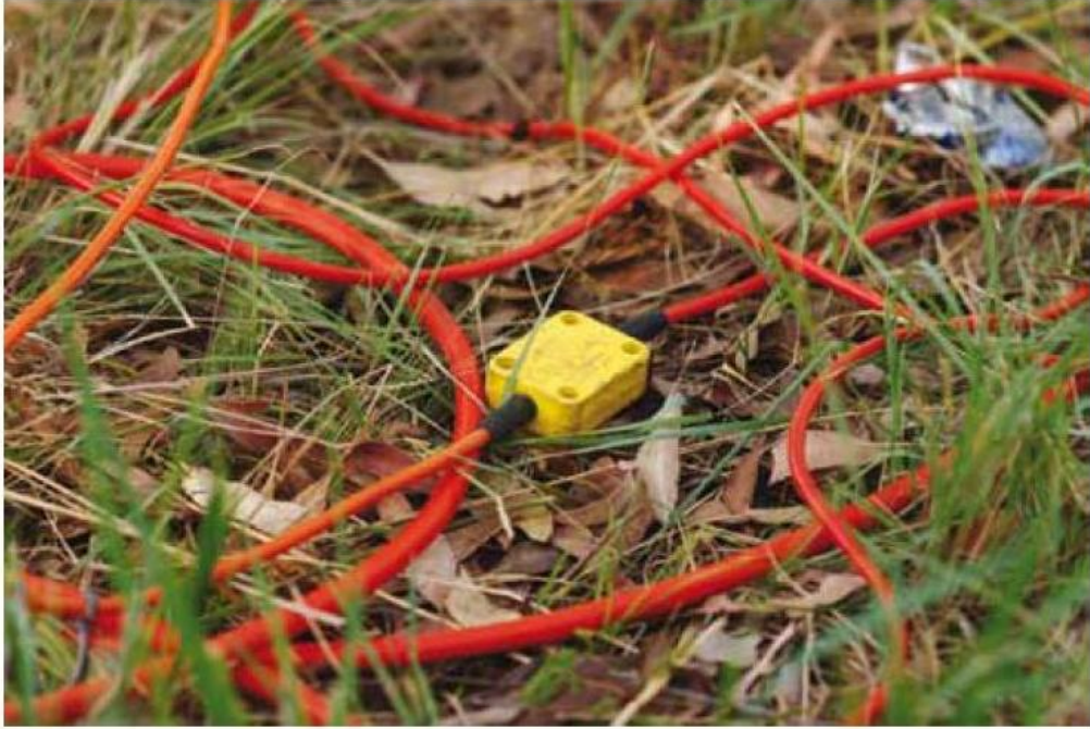
Figure 26 Geophone receiver setup on surface. (AGL)
