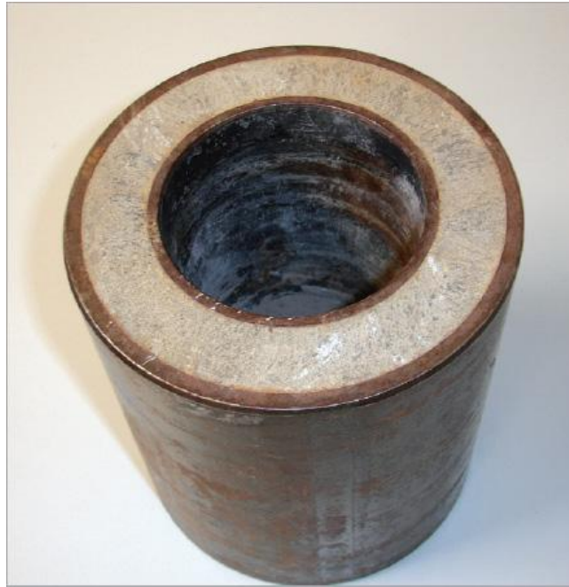
Figure 31 Cross section of double steel casing (AGL).
