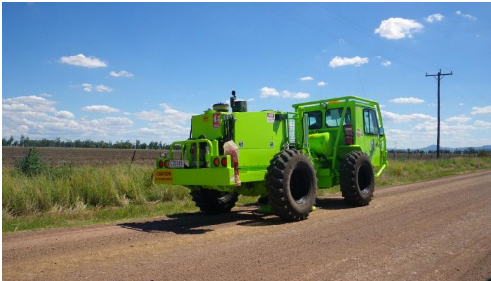
Figure 25 Basic seismic surveying vehicle (Arrow Energy)
