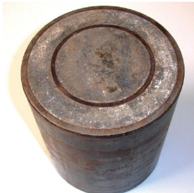
Figure 32 Cross section of abandoned double steel casing (AGL)
