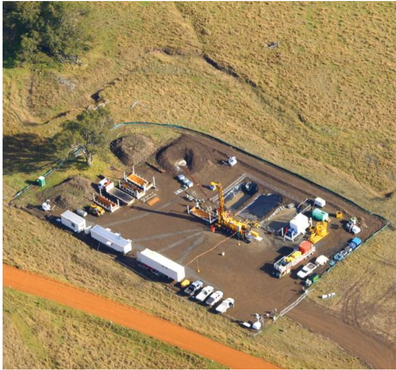
Figure 28 Typical core hole drilling site (Santos)
