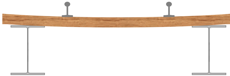
Figure 3.1.8. Eccentric loading causing the transoms to load the inside edge of the top flange.
