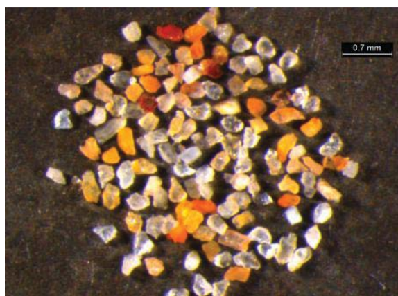
Figure 4-2. A K-rich feldspar aliquot from sample KHUT-1 containing a mixture of K-rich feldspar, quartz, plagioclase and possibly other minerals. Sodium polytungstate ( \rho < 2.58 \text{ g/cm}^3 ) was used to remove quartz, plagioclase and heavy minerals from the 180–212 \mu\text{m} grain size fraction. The separate was then etched for 10 min with a diluted HF acid (10%) solution. The microphoto was taken using a digital camera mounted on a Leica MZ16A stereo microscope.
