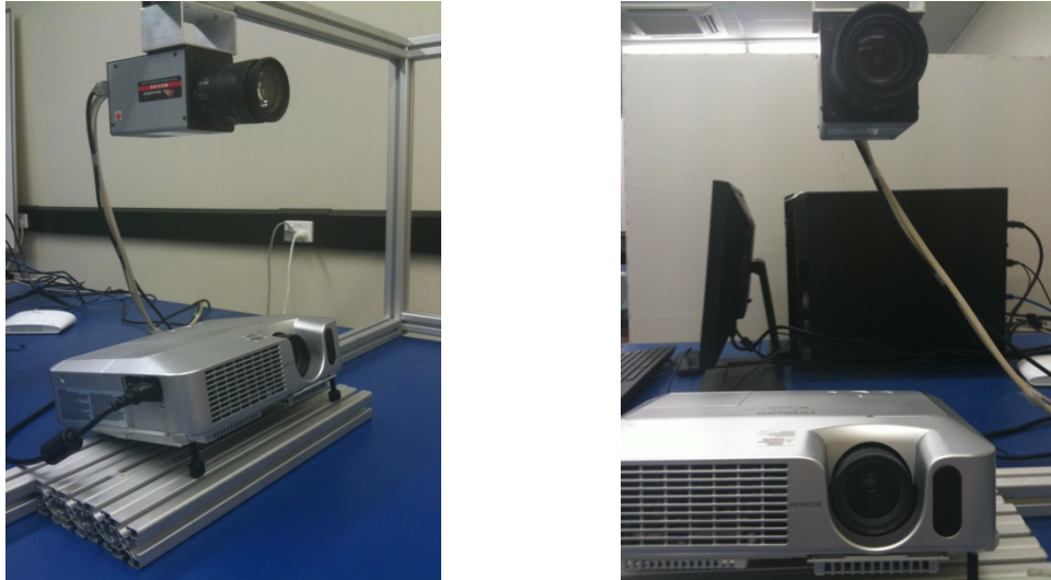
Figure 3.7: Position between the camera and the projector (camera on the top and projector on the bottom).
