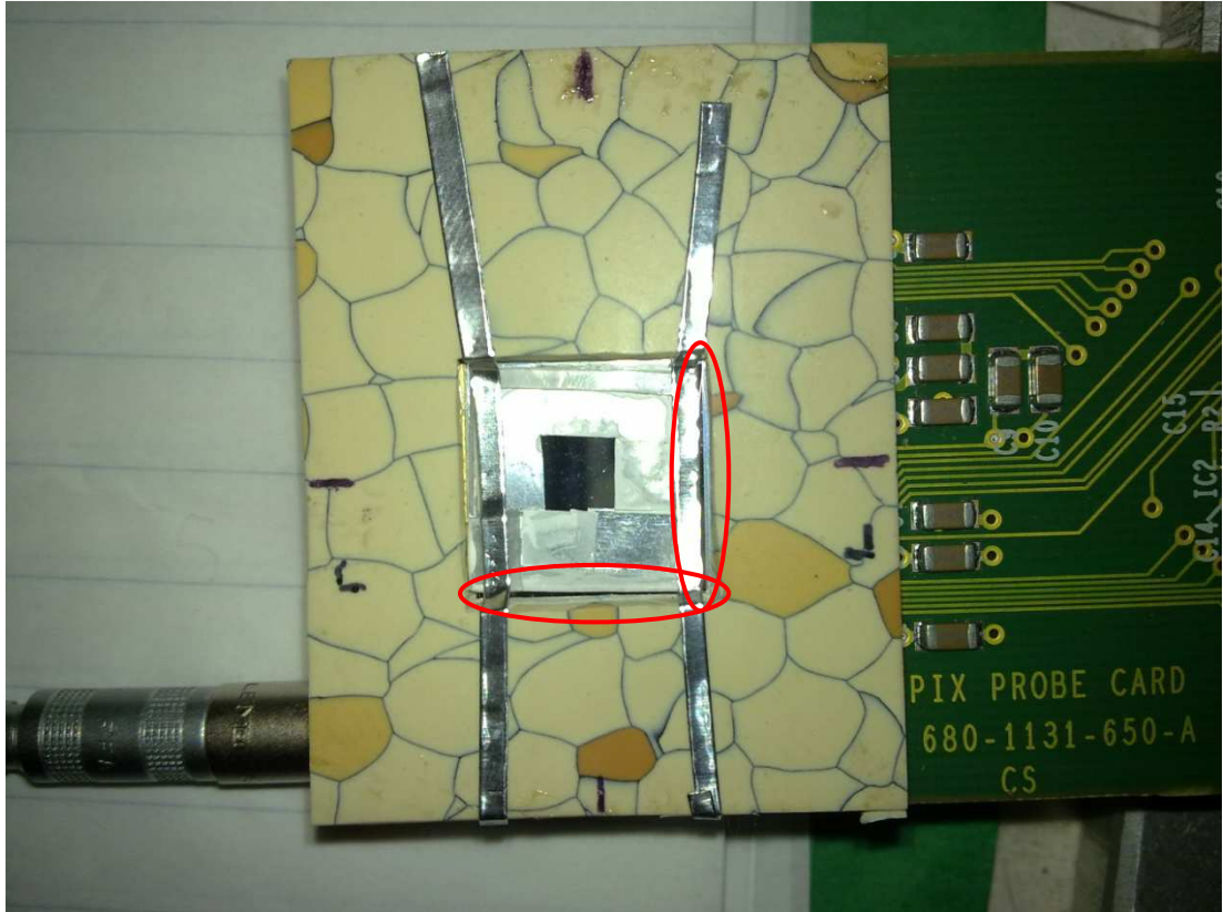
Figure 6.14: Medipix2 with a structured converter attached onto the sensor. A small twist on the converter, which occurred when it was being installed on the Medipix2, may have uncovered the periphery of the sensor (as indicated by the red circles).
