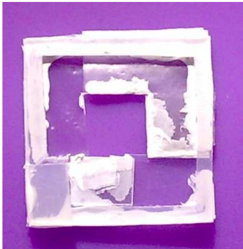
Figure 6.13: The structured polyethylene converter as described in Figure 6.10. The white region is the thin layer of hydrogen-free glue; protons generated from the glue can be neglected.
