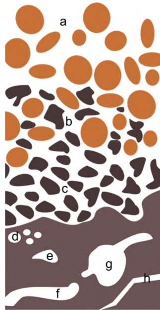
Figure 11.2. Void descriptions based on Stoops (2003). a) simple packing voids; b) complex packing voids; c) compound packing voids; d) vesicles; e) vughs; f) channels; g) chamber; and h) plane. Here, coarse grains are represented in orange, porous crumb as dark brown and micromass as light brown.
