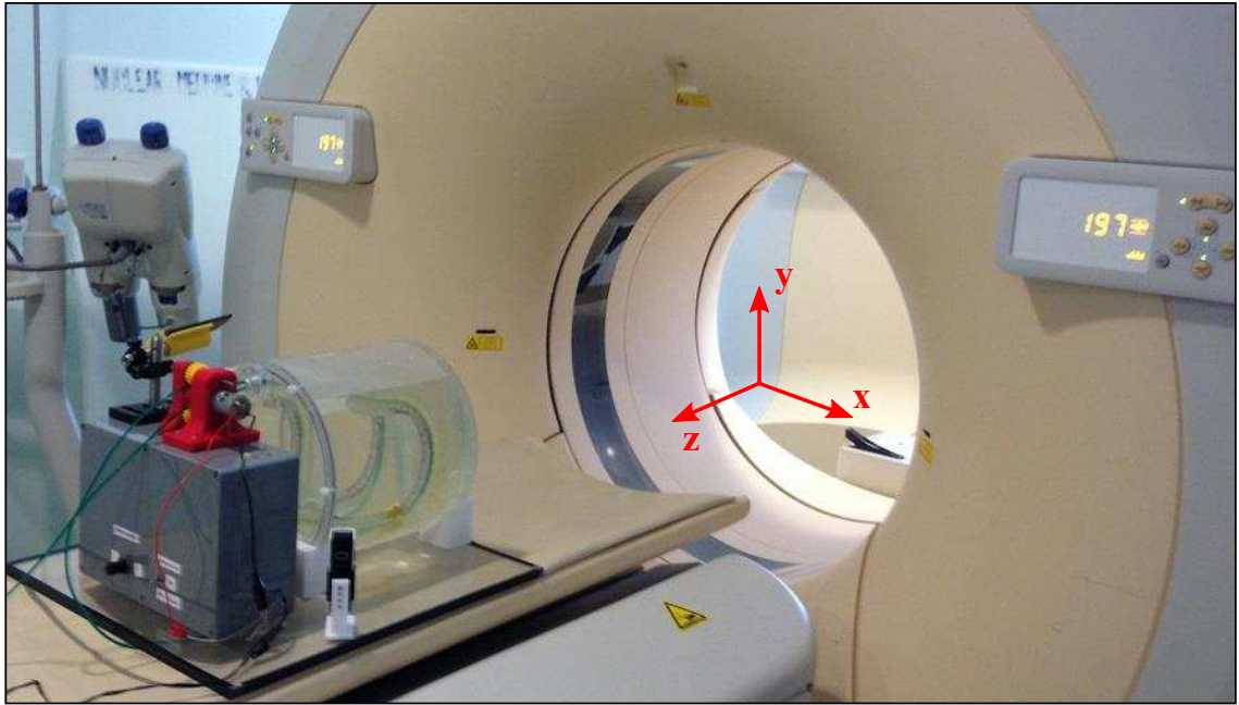
Figure 5.4: The experimental apparatus was placed on the patient bed of a Philips TF64 PET scanner before being moved to the centroid for scanning
