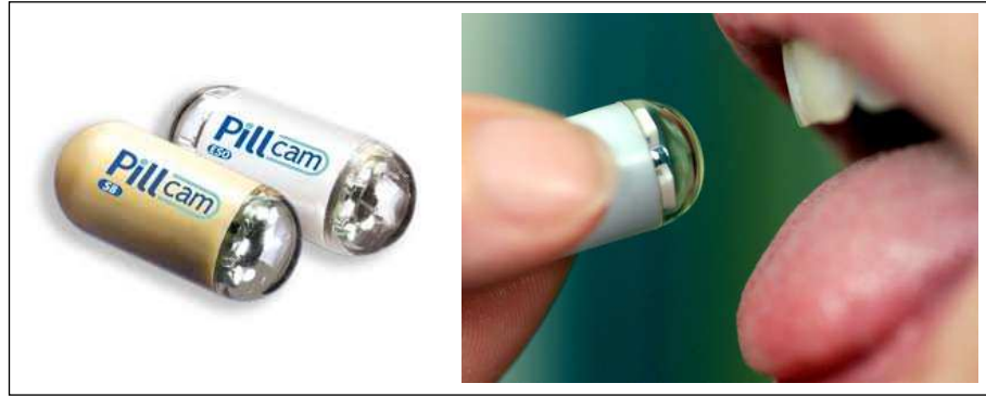
Figure 1.2: Pillcam endoscopic capsules and their small size that makes them swallowable ( www.thehepcexperiment.com ).
