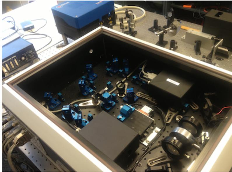
FIGURE 3.8: Photograph of enclosed Zomega TDS system. The femtosecond pump laser is positioned to the top of the photograph.
