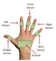
Figure 7. Position of the feedback electrodes.
