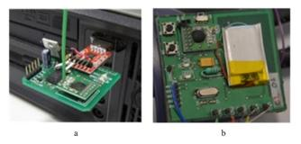
Figure 6. a.USB transmitter b.TENS receiver unit.
