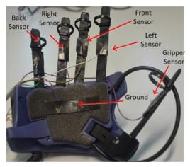
Figure 5. TENS electrodes fitted to data glove.
