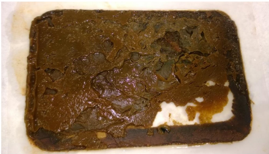
Fig. S1: Photograph of the FO membrane surface at the conclusion of the experiment. Membrane cleaning was not conducted. Experimental condition: CTA-FO membrane; FO mode; draw solution = 1 M NaCl; cross-flow rate = 1 L/min (i.e. cross-flow velocity = 9 cm/s); HRT = 24 h; DO concentration = 5 \pm 1 mg/L; temperature = 22 \pm 1 °C; MF water flux = 1.6 – 2.6 mL/min.
