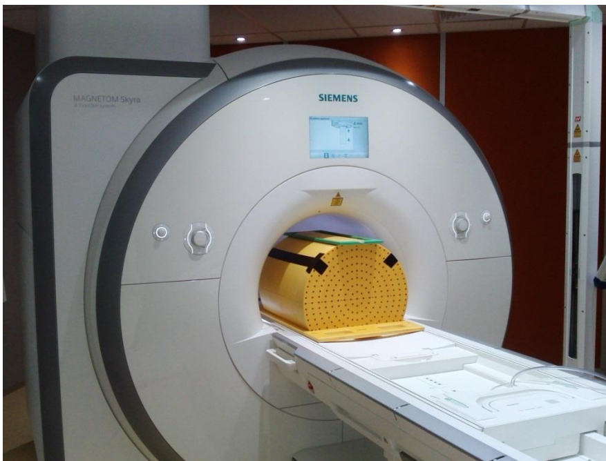
Fig. 1: Photograph of the distortion phantom positioned in a 70 cm wide bore 3 T Siemens Skyra
