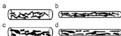
Figure 6. Schematic representation of (a) CNT percolative network relaxed state, (b) CNT percolative network under strain; (c) CNT cluster network relaxed state and (d) CNT cluster network under strain.
