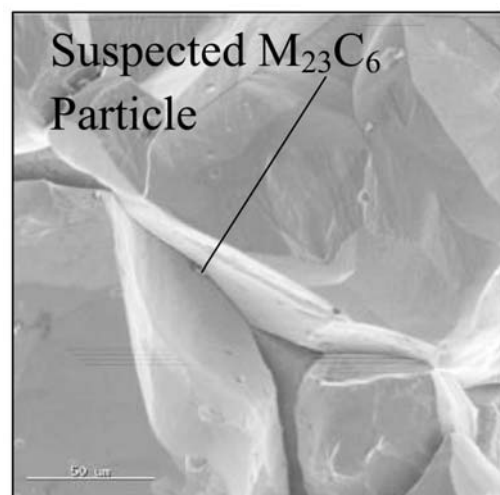
Figure 30—M 23 C 6 on ditched grain boundary after Practice Z (weld heat input—0.8 kJ/mm)
