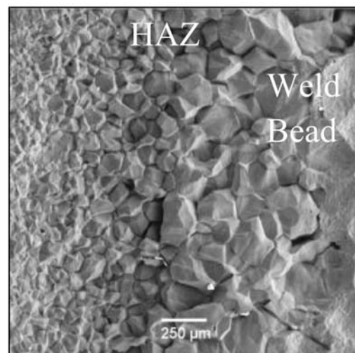
Figure 21—4 mm thick AISI 409 welded at a heat input of 0.32 kJ/mm (Modified Practice Z)
