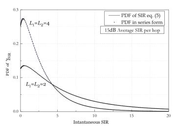
Fig. 2. PDF of destination SIR  $f_{\gamma_{\rm SIR}}\left(\gamma\right)$  as a function of instantaneous SIR.
