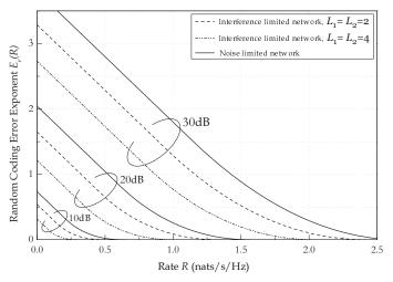
Fig. 3. Random coding error exponent as a function of rate R in nats/s/Hz for different SIRs per hop.
