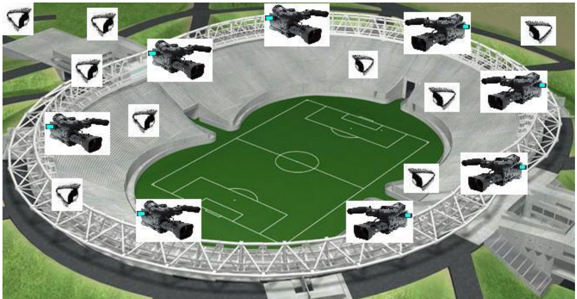
Figure 2.1. Overview of a sample FVV system
