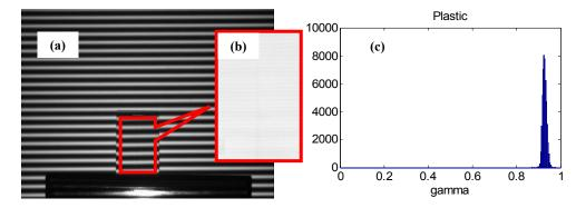
Fig 2. Experiment results for plastic (an access card): (a) the captured fringe image and selected area (marked with red box); (b) the distribution of  $\gamma$  in selected area; (c) the histogram of (b).
