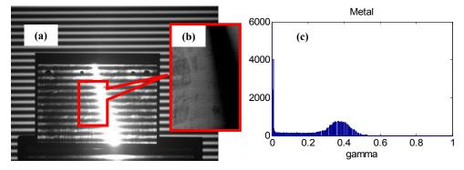
Fig 3. Experiment results for metal (Aluminum alloy): (a) the captured fringe image and selected area (marked with red box); (b) the distribution of  $\gamma$  in selected area; (c) the histogram of (b).
