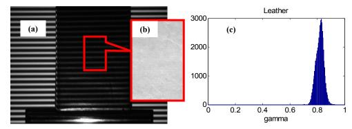
Fig 5. Experiment results for leather (a notebook): (a) the captured fringe image and selected area (marked with red box); (b) the distribution of  $\gamma$  in selected area; (c) the histogram of (b).
