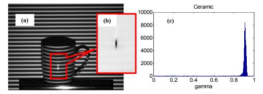
Fig 4. Experiment results for ceramic (a cup): (a) the captured fringe image and selected area (marked with red box); (b) the distribution of  $\gamma$  in selected area; (c) the histogram of (b).
