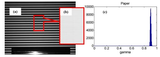
Fig 6. Experiment results for paper: (a) the captured fringe image and selected area (marked with red box); (b) the distribution of  $\gamma$  in selected area; (c) the histogram of (b).
