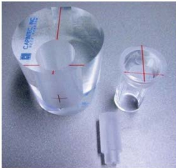
Fig. 2. The Capintex ® thyroid neck phantom made from PMMA provide tissue neck equivalent with 13 cm diameter
