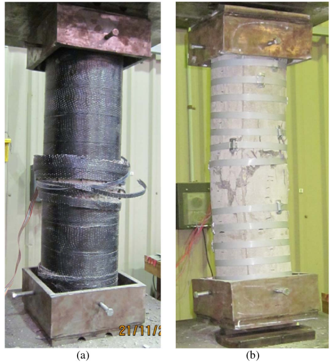
Fig. 9. Failure modes: (a) Specimen CF-0 and (b) Specimen CS-15
