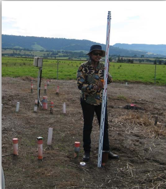
Surveying the piezometers and monitoring wells to locate them in the map and to determine the water table according to AHD
