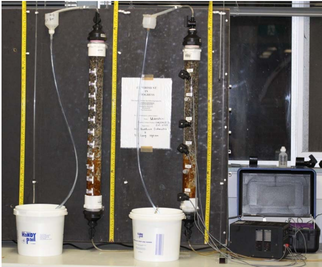
Figure 3.4: Photo of the laboratory column experiments using constant flow method (Left: Sampling column, Right: Pressure transducer column).
