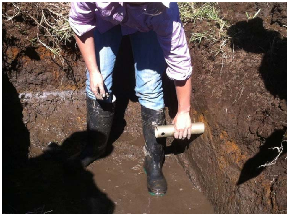
Collecting undisturbed samples of ASS for permeability test
