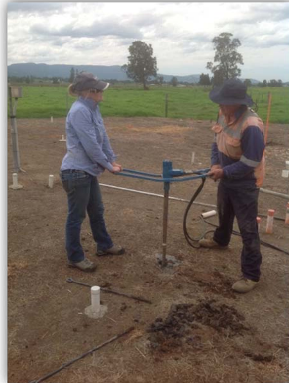
Collecting the bore hole samples using the mechanical auger
