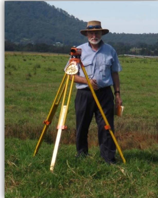
Surveying the piezometers and monitoring wells to locate them in the map and to determine the water table according to AHD
