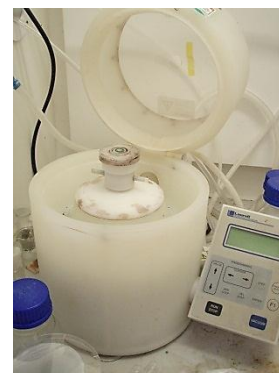
Figure 3.25 – Laurell Ws-400-6npp Lite spincoater.
