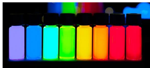
Figure 2.20 – ZnCdSeS quantum dots with various sizes emitting at various wavelength (PlasmaChem).
