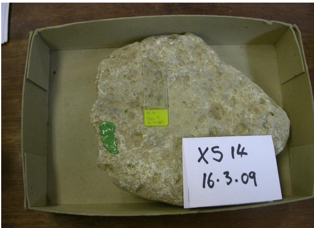
Figure 6: Lower stone XS14 made of tuff showing PVS Peel A (after cleaning and before use).
