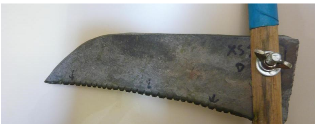
Figure 17: Experimental sickle for harvesting Quercus sp. acorns.
